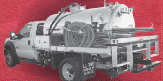
1200 Gallon 2-Compartment Tank (900/300) Mounted On 2012 Ford F550 With Masport Plug & Play Pump
