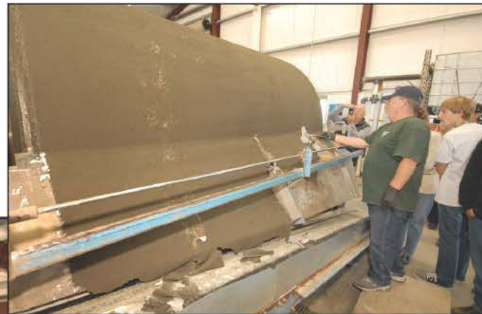
Hess checks the quality of dried solids as they come off the Alar drum.
