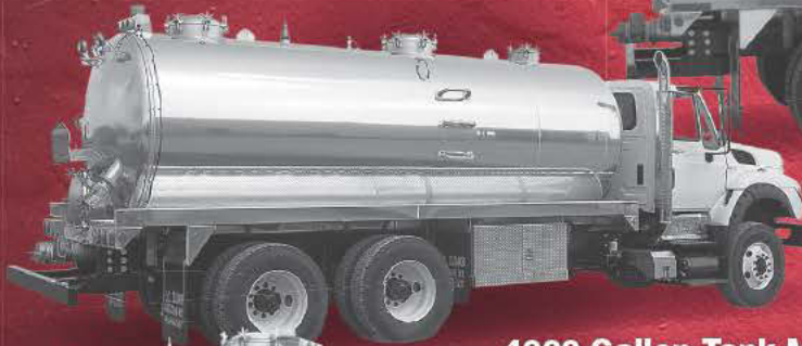
4000 Gallon Tank Mounted On 2011 IH 7600 With NVE 866 Pumping System
