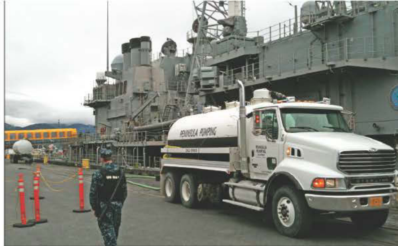
A pumping rig is used in tandem with a pup trailer to offload waste from a U.S. Navy ship stopping at a local dock during military exercises.
