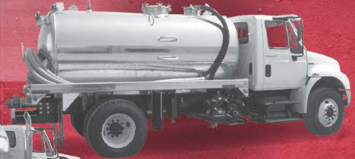
1850 Gallon Septic Pumper Mounted On 2012 IH Chassis
