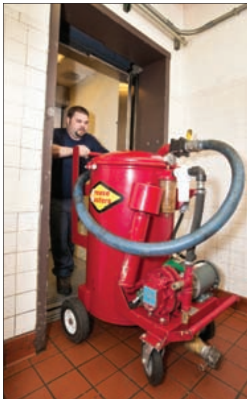
Jeremiah Burpo maneuvers a tight kitchen space with the Dyna-Lite (left), then gets to work emptying the grease trap.
