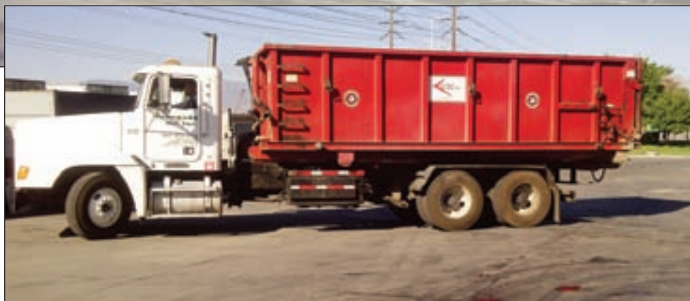
Above is an array of cone-bottom settling tanks used by Renegade to process and store recycled yellow grease and waste vegetable oil. Below is a truck-mounted Flo-Trend 40-cubic-yard Sludge Mate dewatering system. The tank acts as a fill and settle box, with sludge hauled to a transfer station. (Photos courtesy of Renegade Oil)
