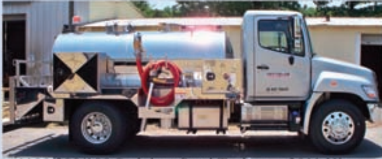
1100/200/100 Stainless Steel Tank on a 2011 Hino truck.
