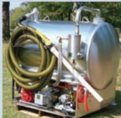
300/110 Stainless Steel Slide In Unit.
