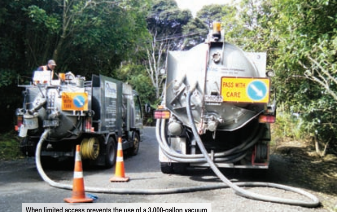
When limited access prevents the use of a 3,000-gallon vacuum truck, a smaller unit is used. Here, the smaller rig transfers a load to the bigger truck for transport to the treatment plant.
