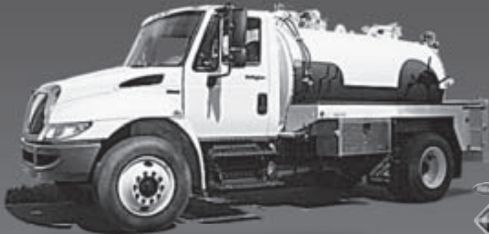
NEW 2012 International, auto trans., 26,000 GVW, 1500 gallon porta jon service unit, Masport HXL75V pump
