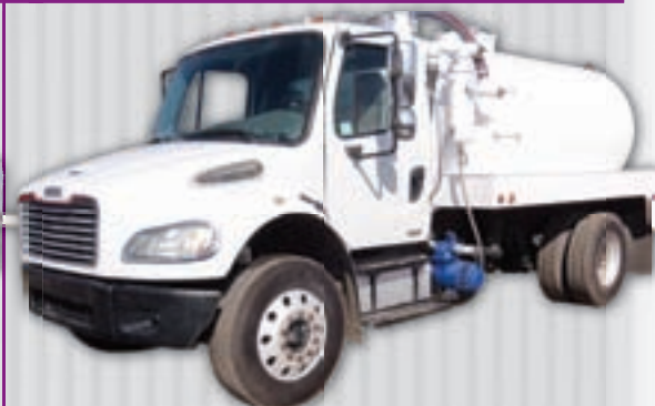
2007 Freightliner M-2 , Cat 300 HP, 9 spd, AC, 33# GVW, new 2300 gallon steel vac tank, new Jurop PN-84 vac pump.
