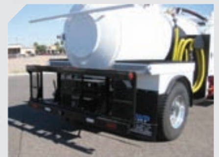
Hotdog style carbon steel waste tank with stainless steel internal tank and convenient dual side service.
