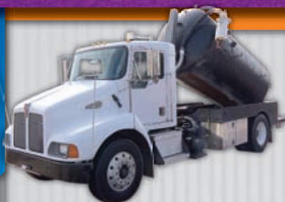
1998 Kenworth T-300 , Cummins 250 HP, 6 spd, AC, 2000 gallon hoist vac tank, NVE 367 Challenger vac pump 36" rear door, jetter pump and reel.
