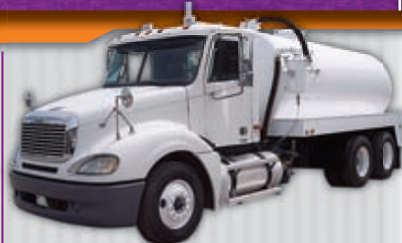
2004 Freightliner Columbia , Detroit 430 HP, 10 spd, jakes, AC, low miles, double framed, new 3360 gallon steel vac tank, new liquid cooled HXL-400 Masport vac pump.
