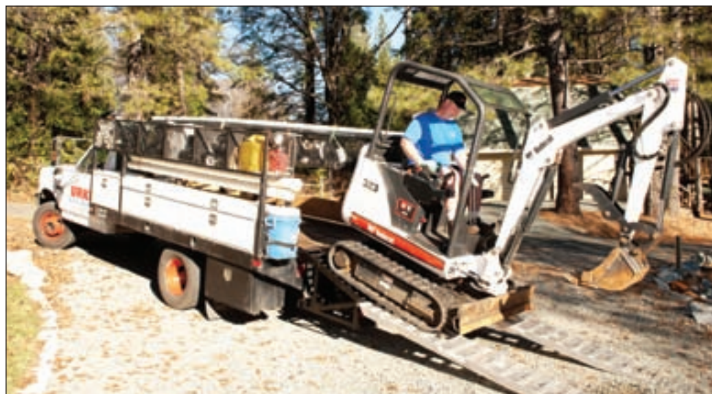
At left, Doug Urke unloads his Bobcat mini-excavator to excavate a septic tank lid for a service call. Above, Bob Zoellin cleans a septic filter.
