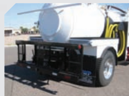
Hotdog style carbon steel waste tank with stainless steel internal tank and convenient dual side service.
