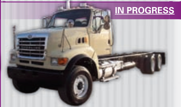
2005 Sterling LT9522 , Cat 350HP, 10spd, 20# fronts, 40# rears on Hendrickson, AC, double framed, new 4000 gallon steel vac tank, new liquid cooled HXL-400 Masport vac pump.
