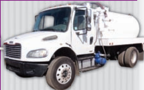
2007 Freightliner M-2 , Cat 300 HP, 9 spd, AC, 33# GVW, new 2300 gallon steel vac tank, new Jurop PN-84 vac pump.
