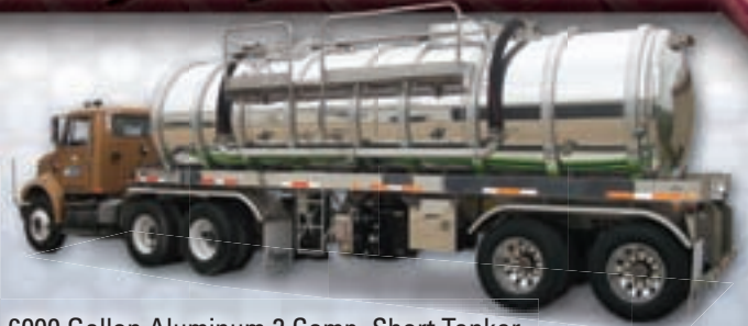
6000 Gallon Aluminum 2 Comp. Short Tanker w/ NVE 866 "Max Pack" Pump System
