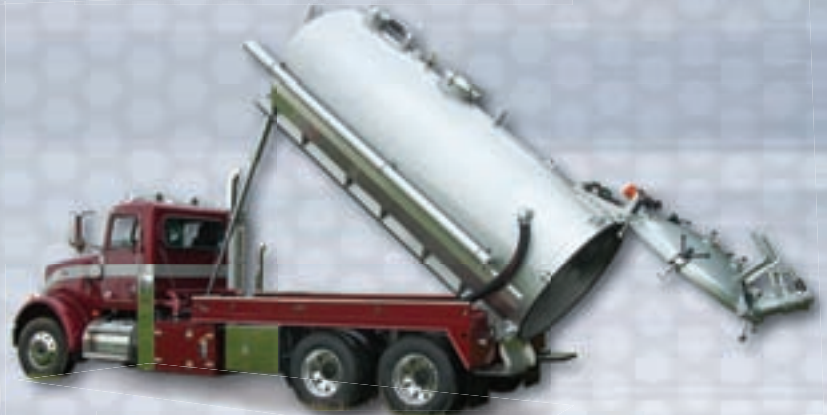
3500 Gallon Aluminum Hoist & Rear Door w/ NVE "Pro-Pack" Blower System
