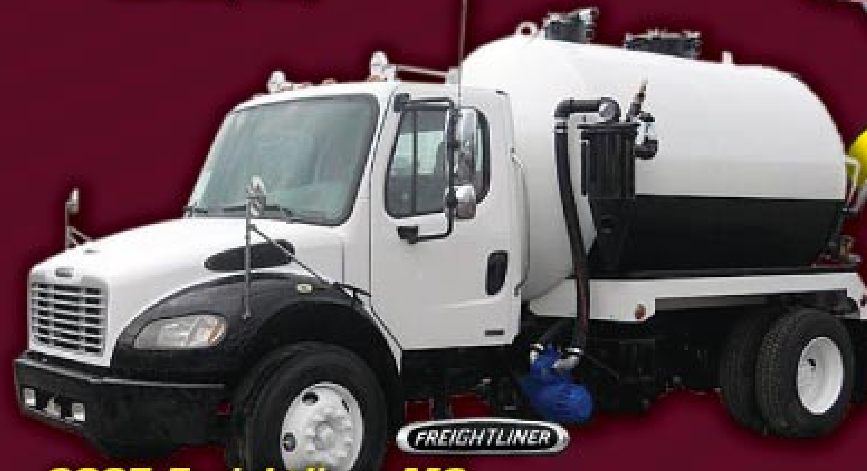
2007 Freightliner M2, Cat Engine, 6-Spd, 2500 Gallon Carbon Steel Tank, Jurop Pump.
