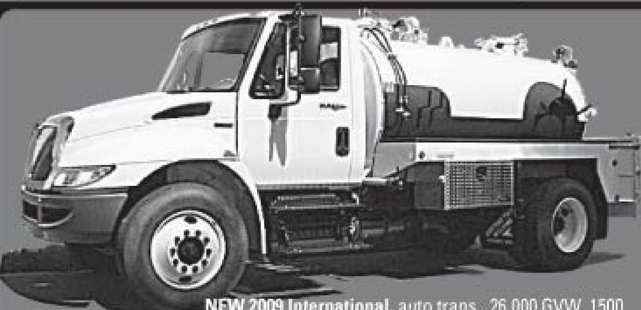
NEW 2009 International, auto trans., 26,000 GVW, 1500 gallon porta jon service unit, Masport HXL75V pump
