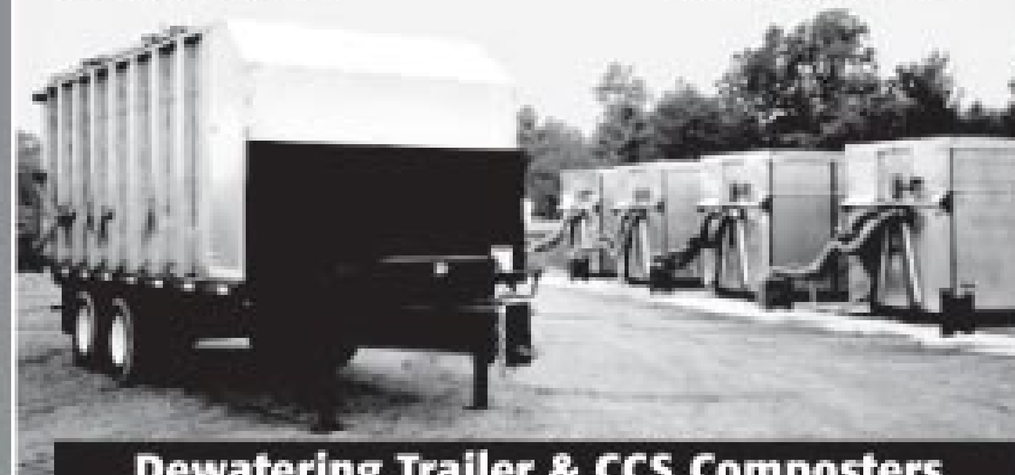
Dewatering Trailer & CCS Composters
