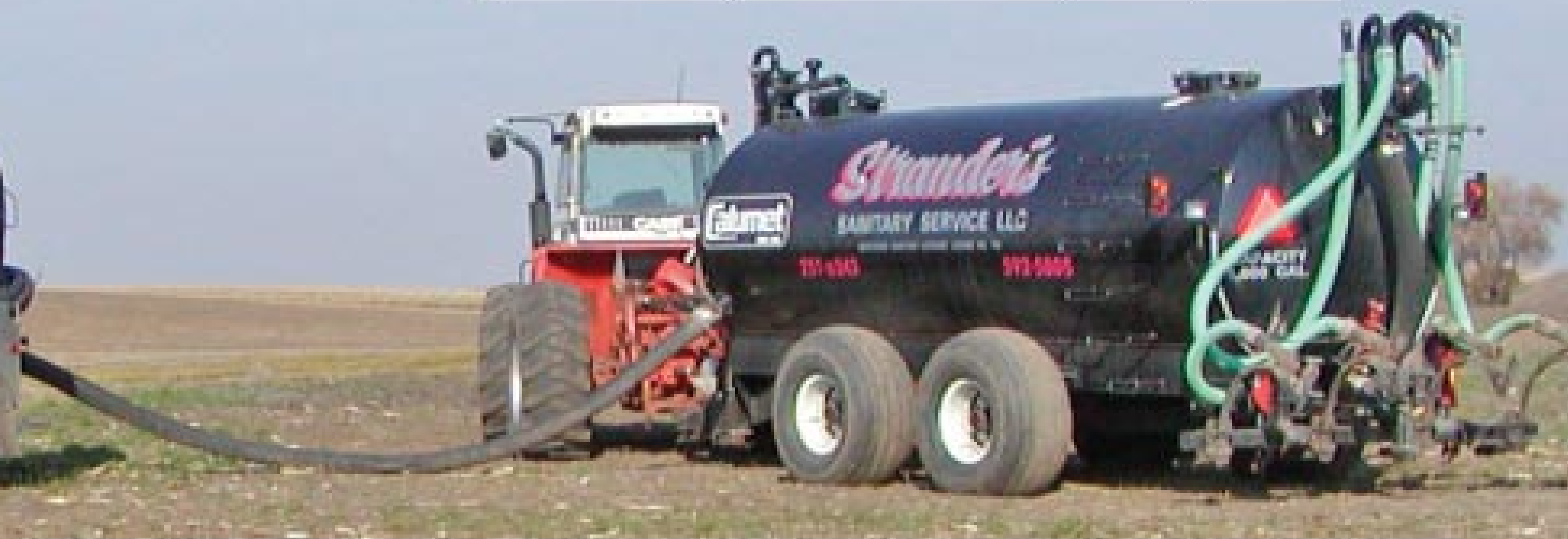
Technicians transfer septage from a vac truck to a 5,000-gallon injector and tractor rig for land application. (Photos courtesy of Strander's Sanitary Service)
