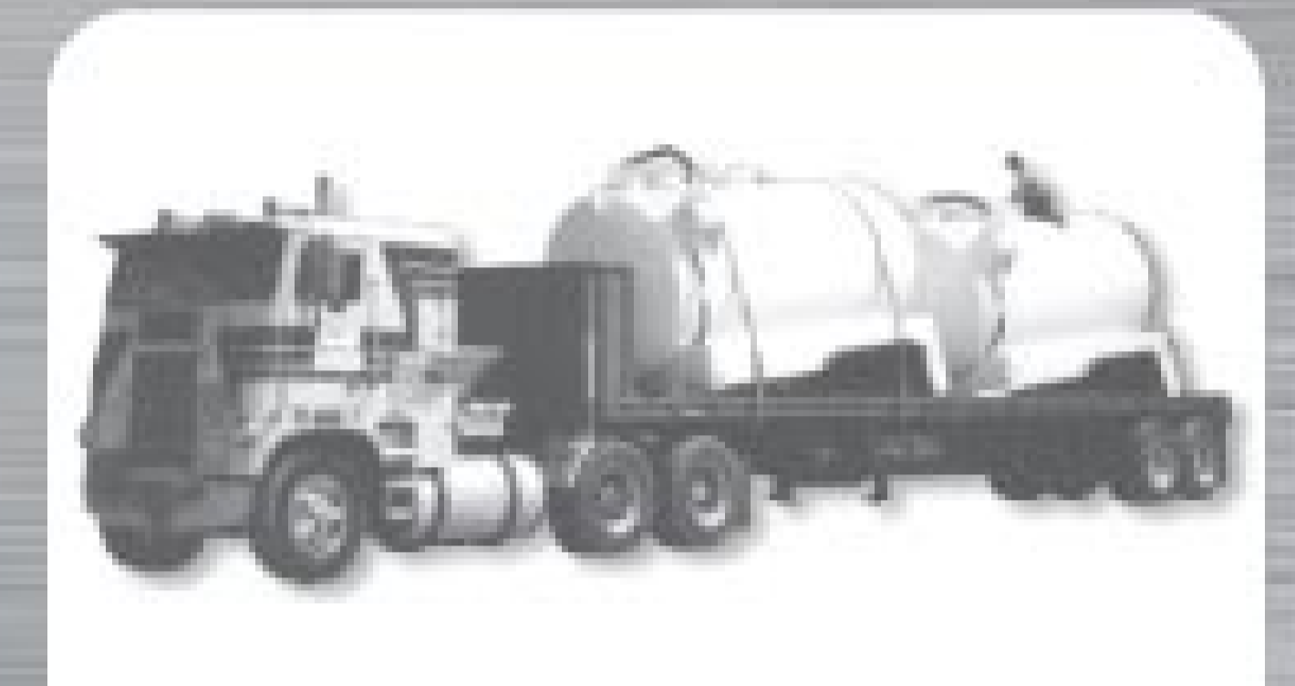
1989 Chevrolet C70, 8.2 ltr. diesel, 5+2 air brakes, double frame, MEC 5000 vacuum pump, 1500 gallon vacuum tank.
