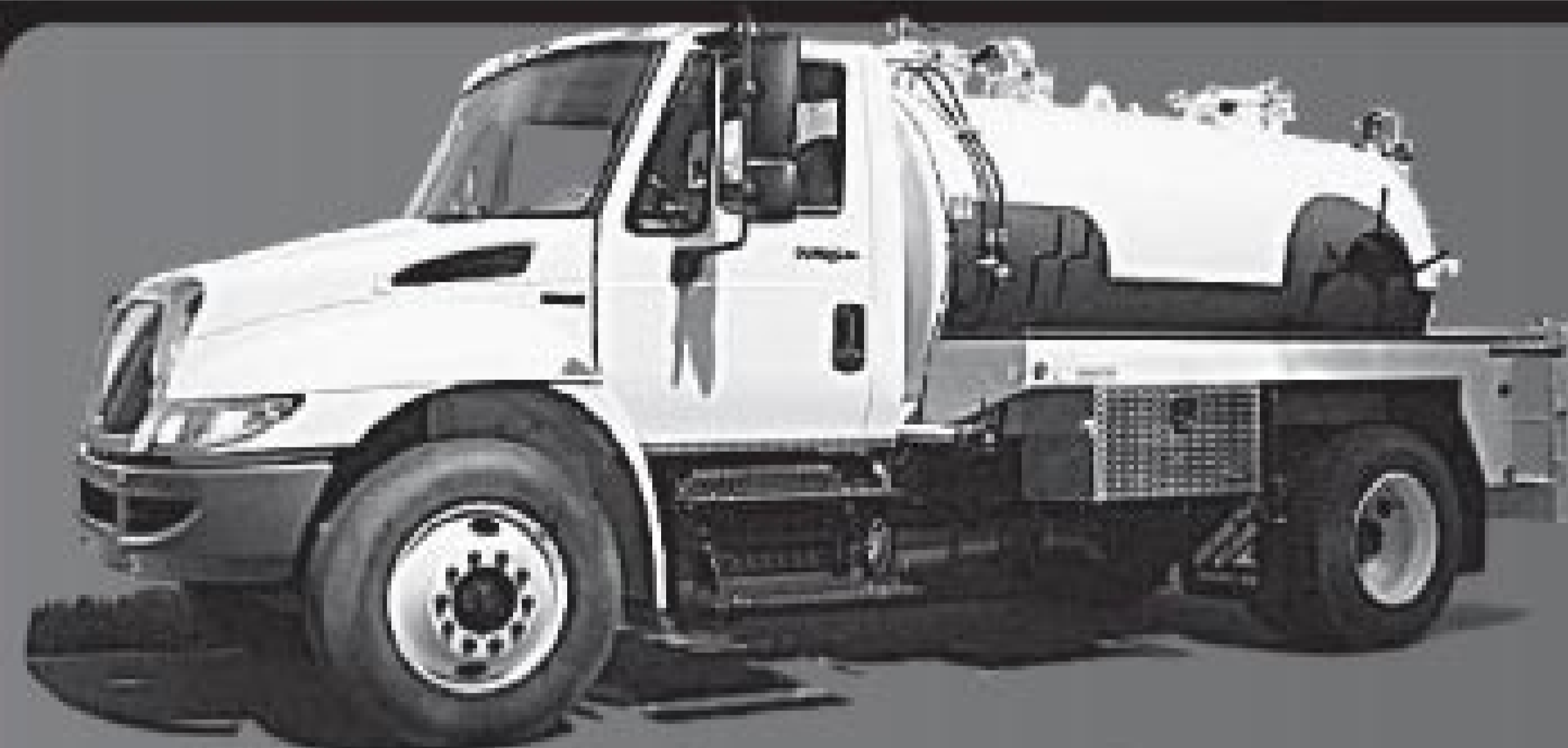
NEW 2009 International, auto trans., 26,000 GVW, 1500 gallon portable service unit, Masport HXL75V pump
