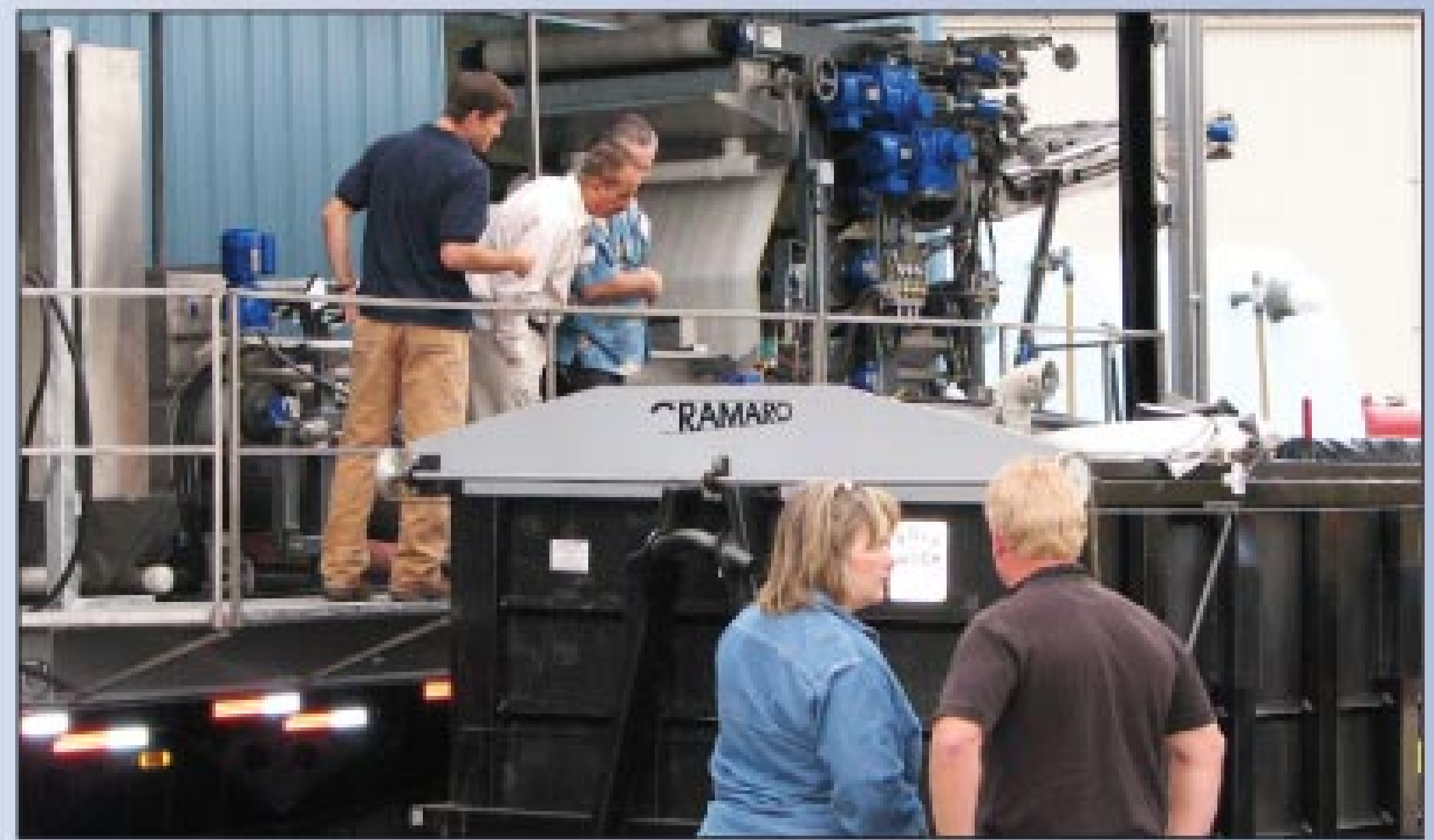
A BDP Industries belt filter press and PolyWick dewatering container processed actual waste at the vendor displays.
