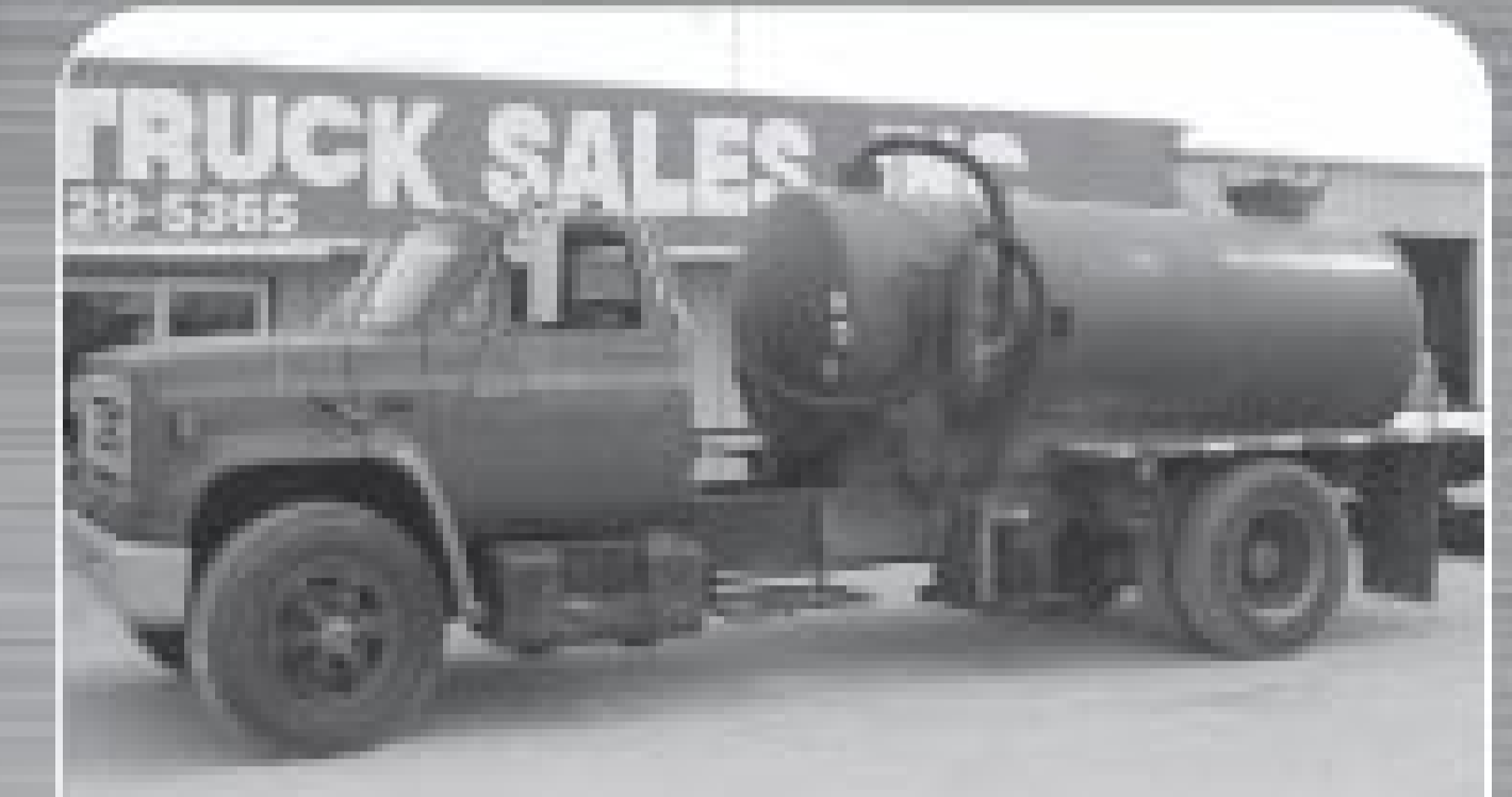
1989 Chevrolet C70, 8.2 ltr. diesel, 5+2 air brakes, double frame, MEC 5000 vacuum pump, 1500 gallon vacuum tank.
