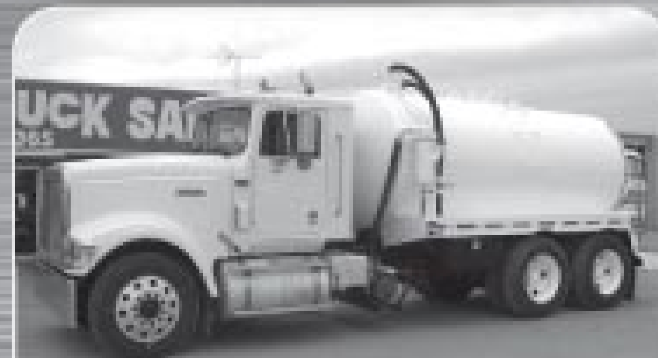
1999 IH 9900, Detroit 60 series (430/500 hp), 10-spd., new Wally 753LN vacuum pump, new 3000 gallon vacuum tank.
