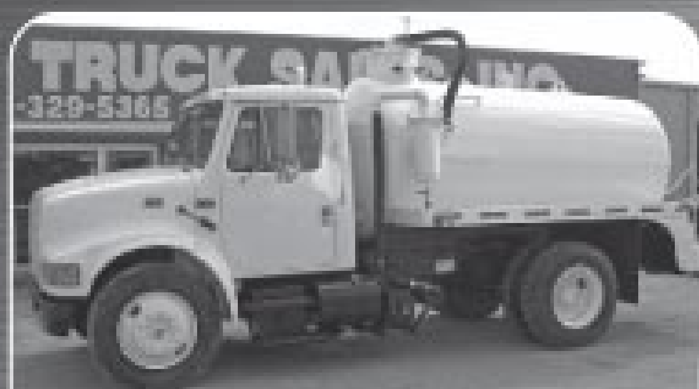
1998 IH 4700, DT466E, 6-spd., double frame, MEC8000/PAL vacuum pump, 1600 gallon vacuum tank.
