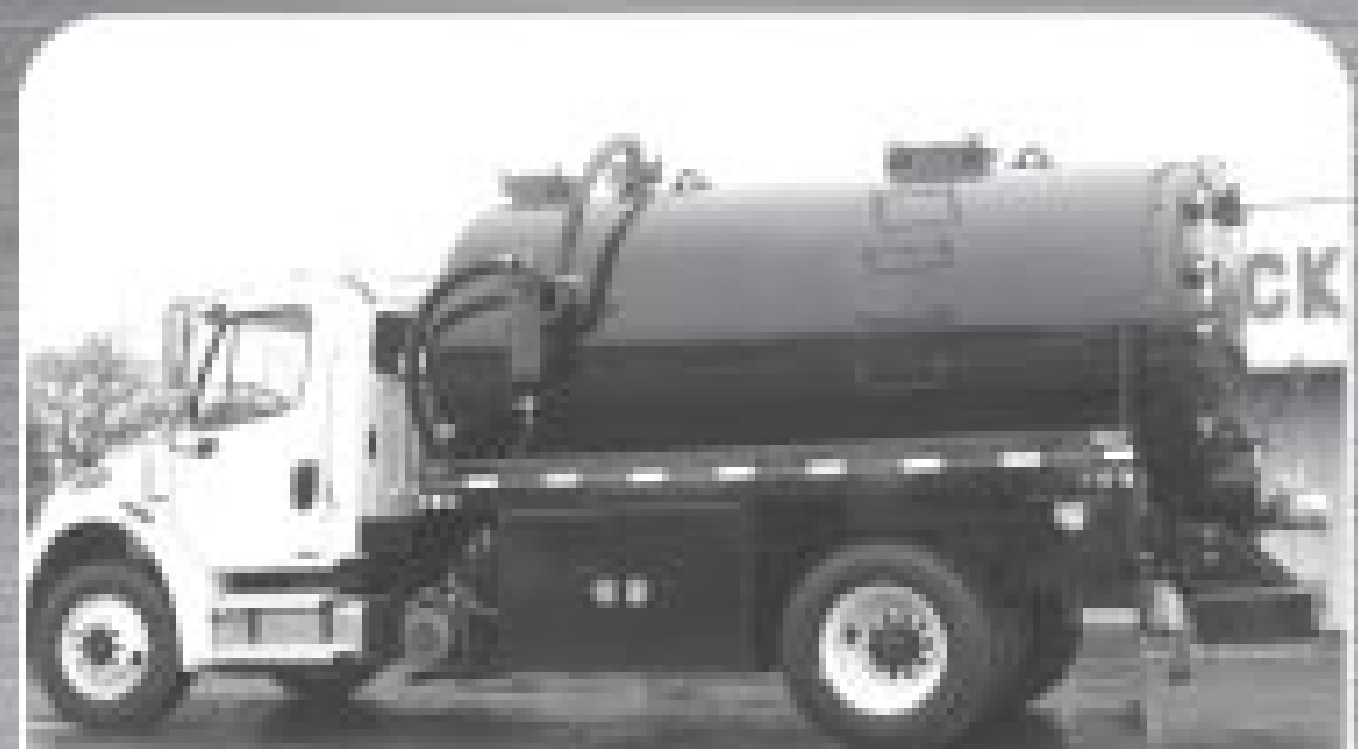
1998 IH 4700, DT466E, 6-spd., double frame, MEC8000/PAL vacuum pump, 1600 gallon vacuum tank.
