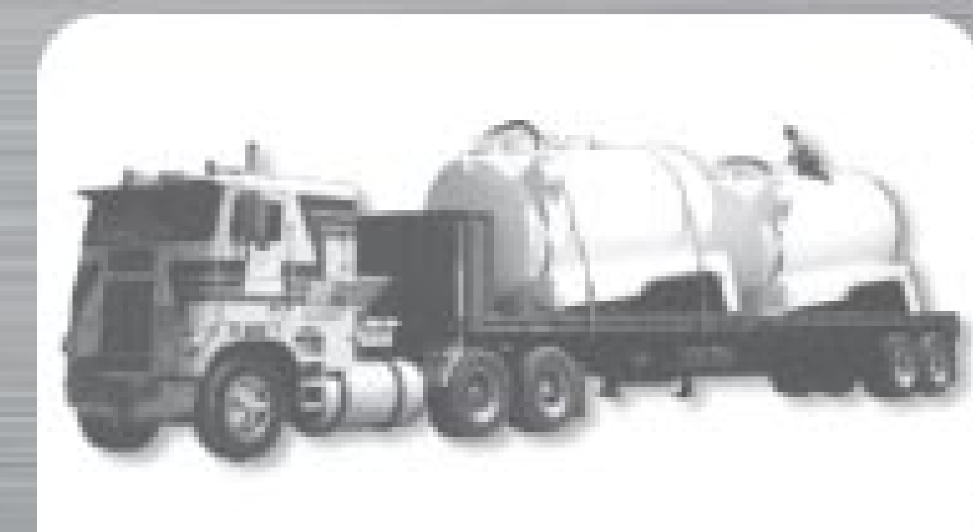
1989 Chevrolet C70, 8.2 ltr. diesel, 5+2 air brakes, double frame, MEC 5000 vacuum pump, 1500 gallon vacuum tank.
