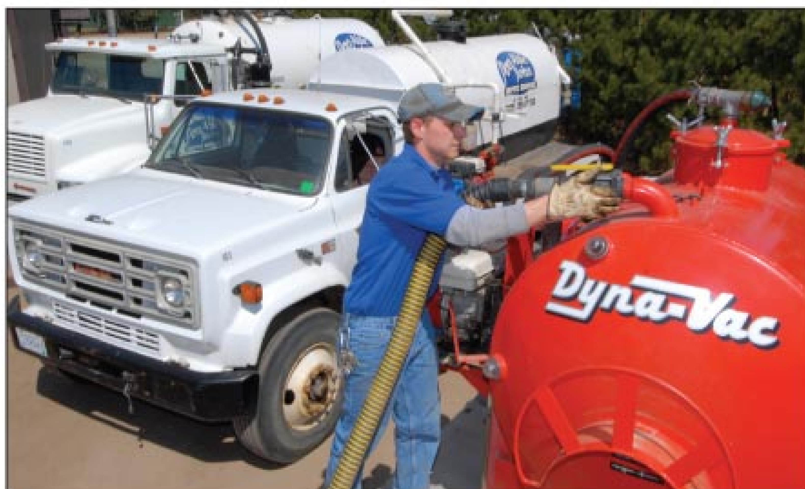
Nathan Johnson attaches a hose coupler to a Dyna-Vac slide-in vacuum tank unit.
