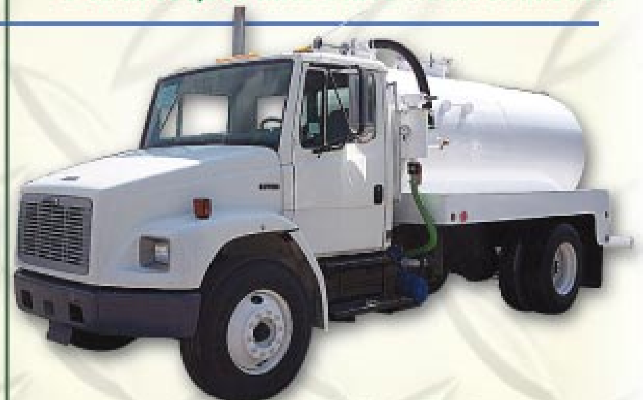
2003 Freightliner FL-70 , Cat 250 HP, 6 spd, AC, 33# GVW, new 2300 gallon steel vac tank, new Jurop PN-84 vac pump. Call For Pricing! 2-YEAR 100,000 MILE DRIVE TRAIN WARRANTY
