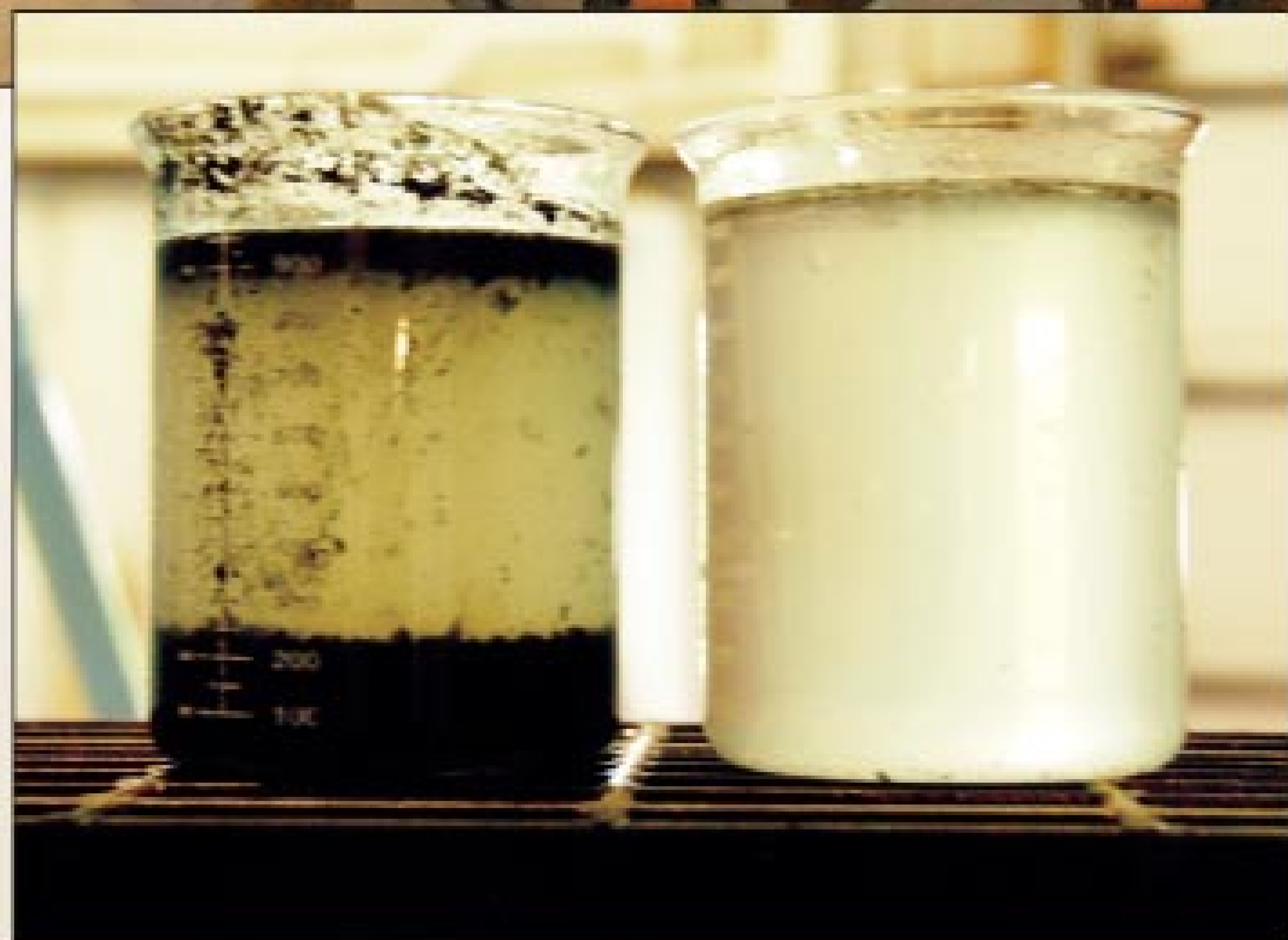
Effluent from the dewatering process has improved with the addition of the PolyWick dewatering box. At left is the decant water from the sludge tanks. At right is the decant water after going through the box built by Bucks Fabricating.
