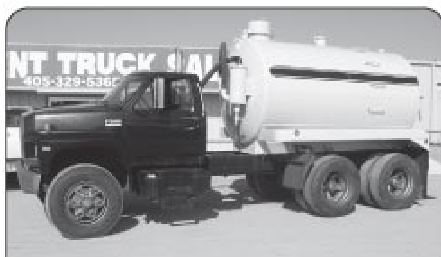
1992 Ford F900, Diesel 210 hp, Allison auto., air brakes, Moro vacuum pump, 2500 gallon vacuum tank.
