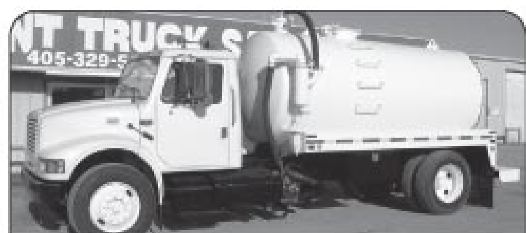
2001 IH 4700, DT466E, Allison auto., non-CDL, 75K miles, new Wally 403HR vacuum pump, new 1600 gallon vacuum tank.
