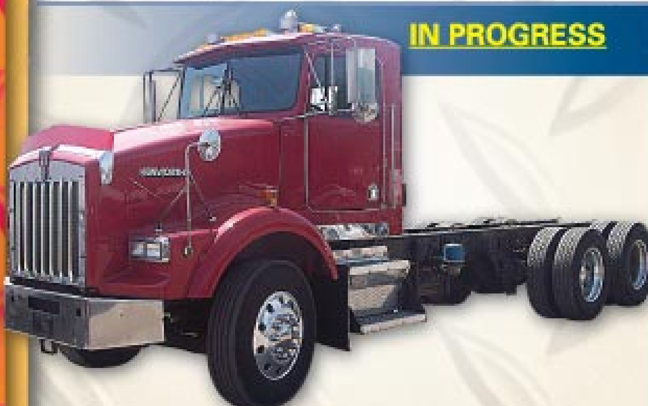
2001 Kenworth T-800 , N-14 Cummins 525HP, 10 spd, jakes, 14,600# fronts, 46# rears, new 3600 gallon steel vac tank, new Masport HXL-400 vac pump. Call For Pricing! 2-YEAR 200,000 MILE DRIVE TRAIN WARRANTY
