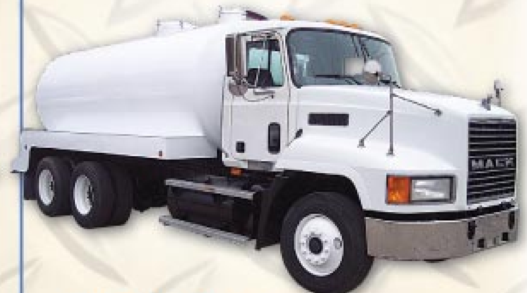
2001 Mack CH613 , E-7 300 HP, 10 spd, AC, double framed, new 3360 gallon steel vac tank, new liquid cooled HXL-400 Masport vac pump. Call For Pricing! 2-YEAR 200,000 MILE DRIVE TRAIN WARRANTY
