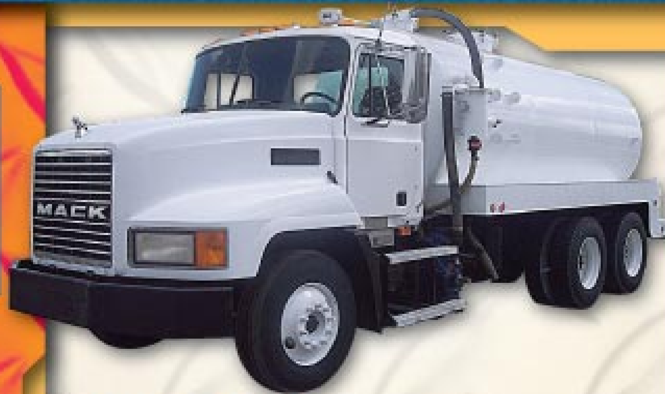
1999 Mack CH613 , E-7 427HP, 10 spd, jakes, AC, 3 year old 3360 gallon steel vac tank, Liquid Cooled HXL-400 Masport vac pump. $41,950
