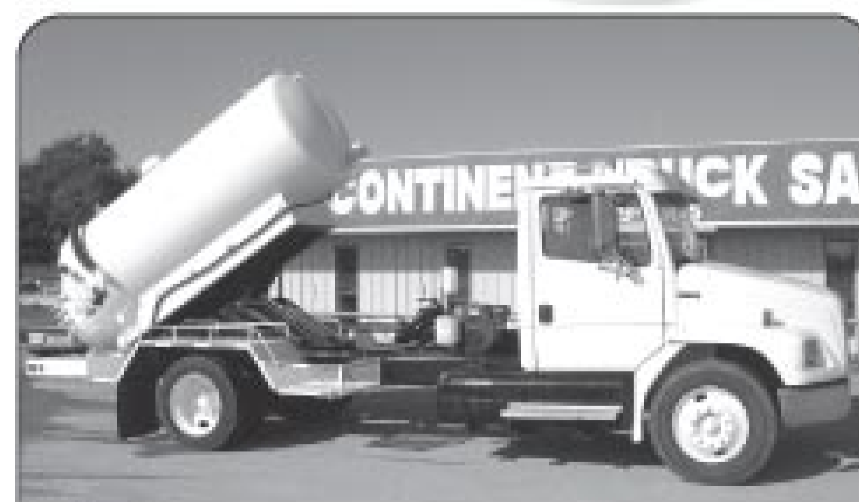
1998 Freightliner FL60, Cummins 5.9 (210 hp), 6-spd., Masport H75V vacuum pump, General 47 series triplex, 1100/200 gallon vacuum tank.
