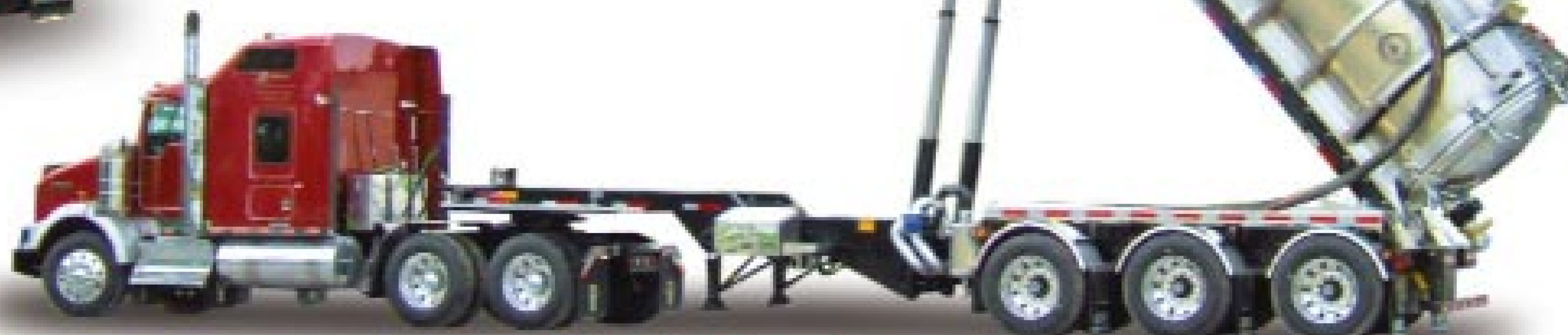
7,150-GALLON ALUMINUM DOT-412 VACUUM DUMPER
