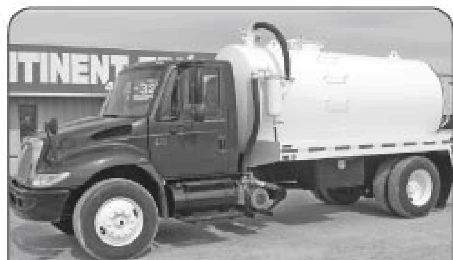
2003 IH 4400, DT466E (215 hp), 6-spd., 33K GVW, new Wally 403HR vacuum pump, new 2300 gallon vacuum tank.
