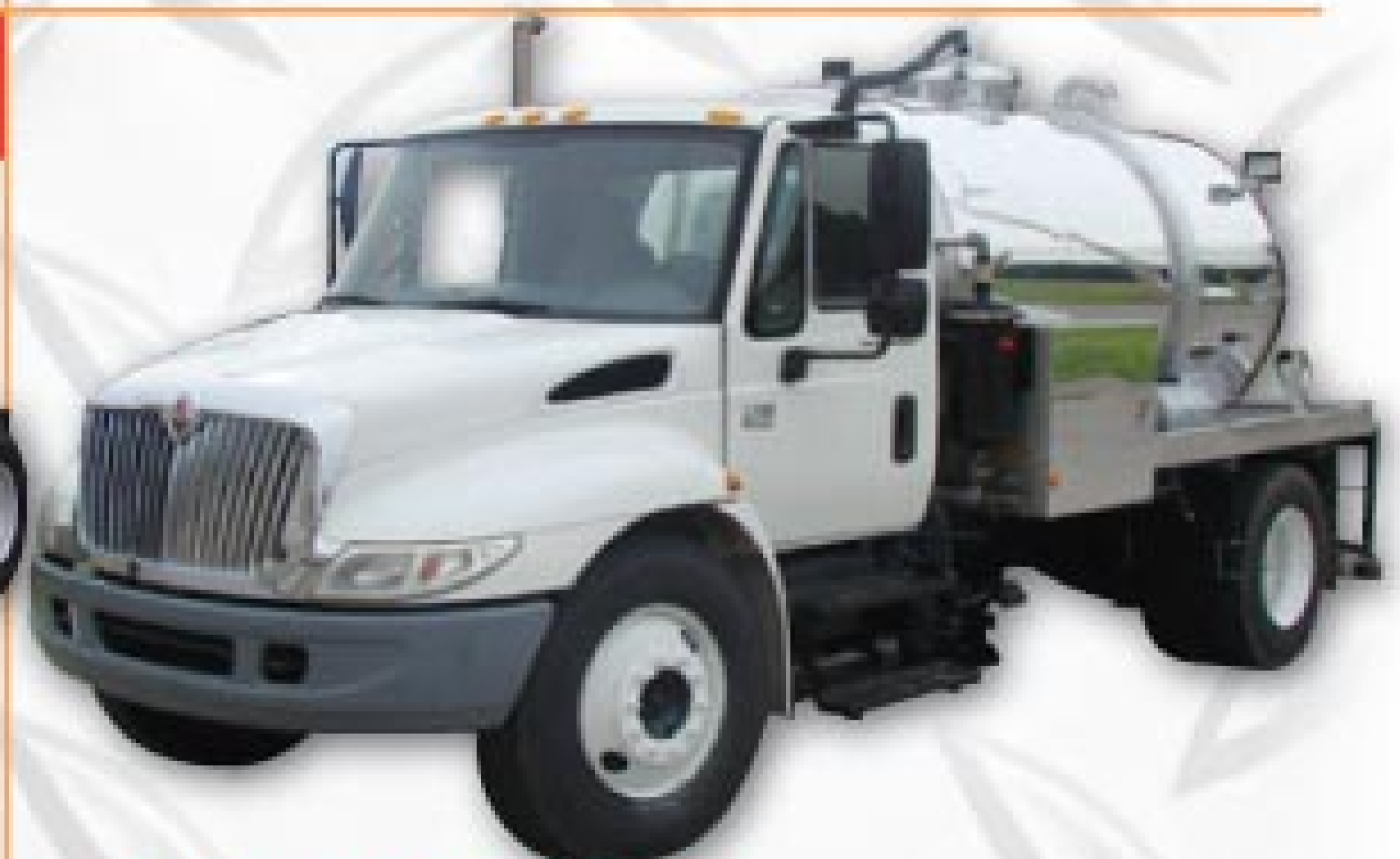
2004 International 4300 , DT-466E 220 HP, Auto, Non CDL, 2000 gallon (500/1500 split) Progress Alum. tank, HXL-75 Masport pump, elec. pressure pump, 4" discharge, portable toilet rack, tank system completely refurbished by Factory, fresh inframe on truck by International $46,800
