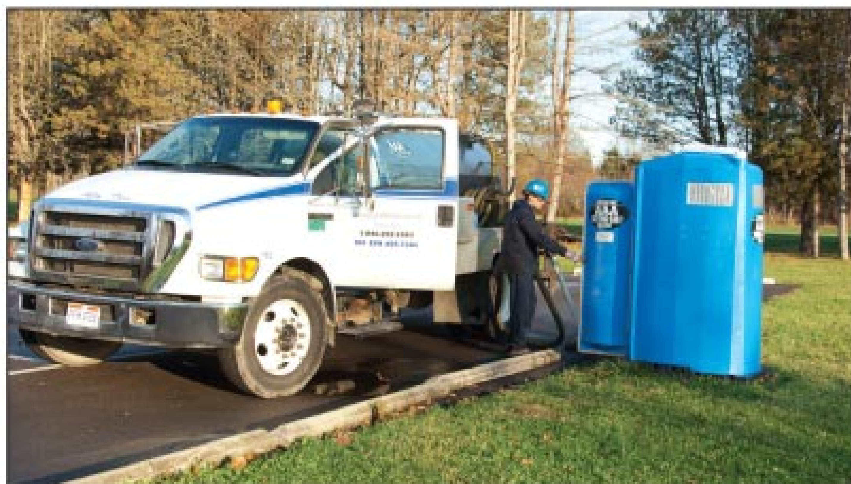
Jeremy Moses vacuums waste from a T.S.F. Tuff Jon portable restroom at a city park into a Ford F-650 service vehicle with 1,200-gallon tank.
