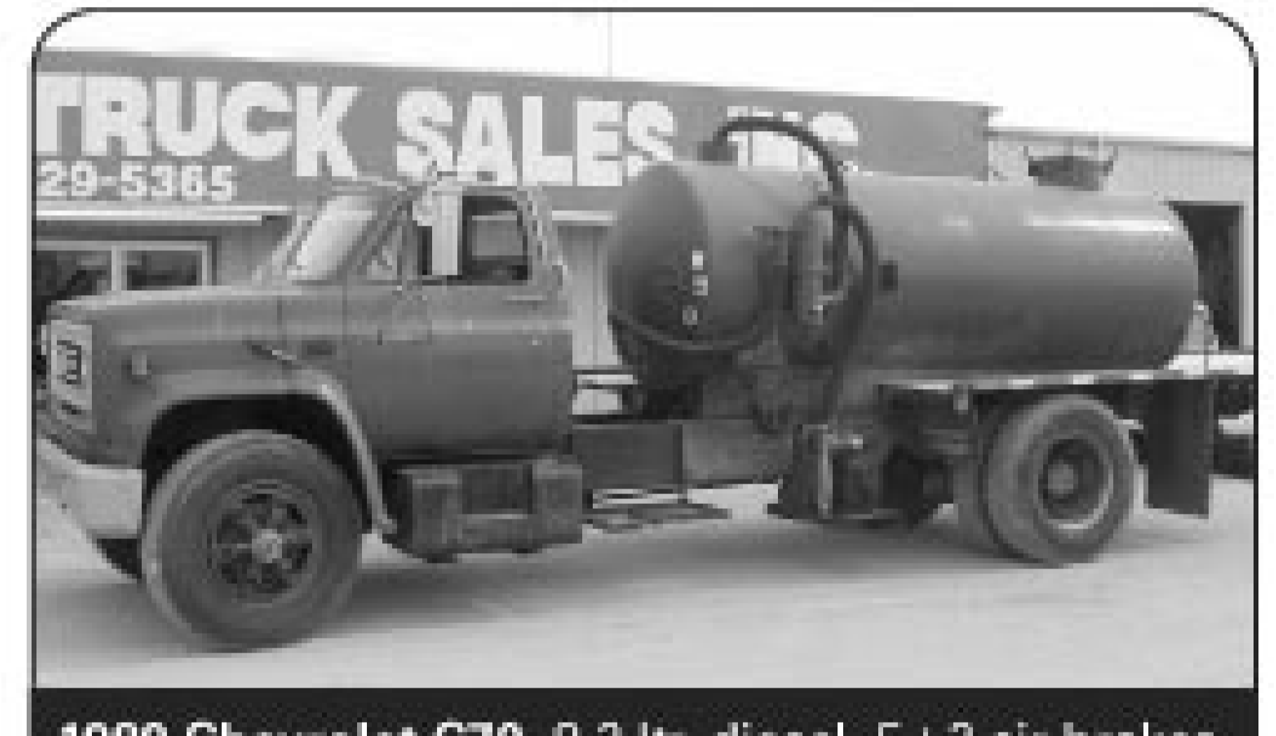
1989 Chevrolet C70, 8.2 ltr. diesel, 5+2 air brakes, double frame, MEC 5000 vacuum pump, 1500 gallon vacuum tank.
