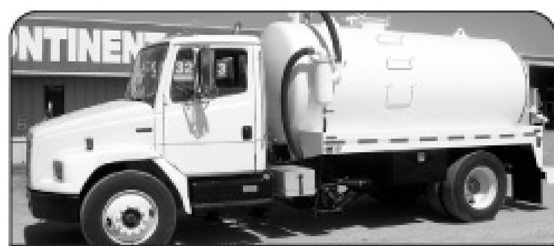
2002 Freightliner FL70, Cat 3126 (210 hp), 6-speed, new Masport HXL75V vacuum pump, new 2300 gallon vacuum tank.
