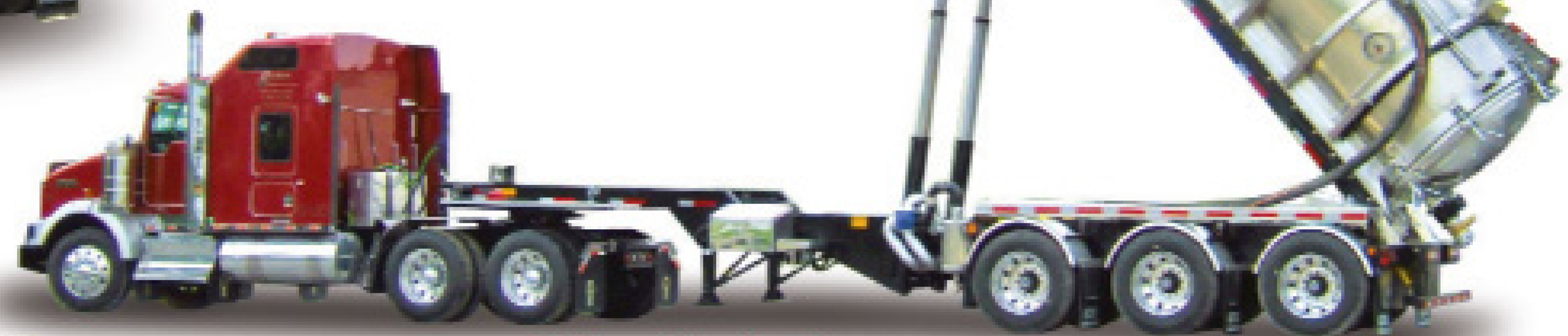
7,150-GALLON ALUMINUM DOT-412 VACUUM DUMPER
