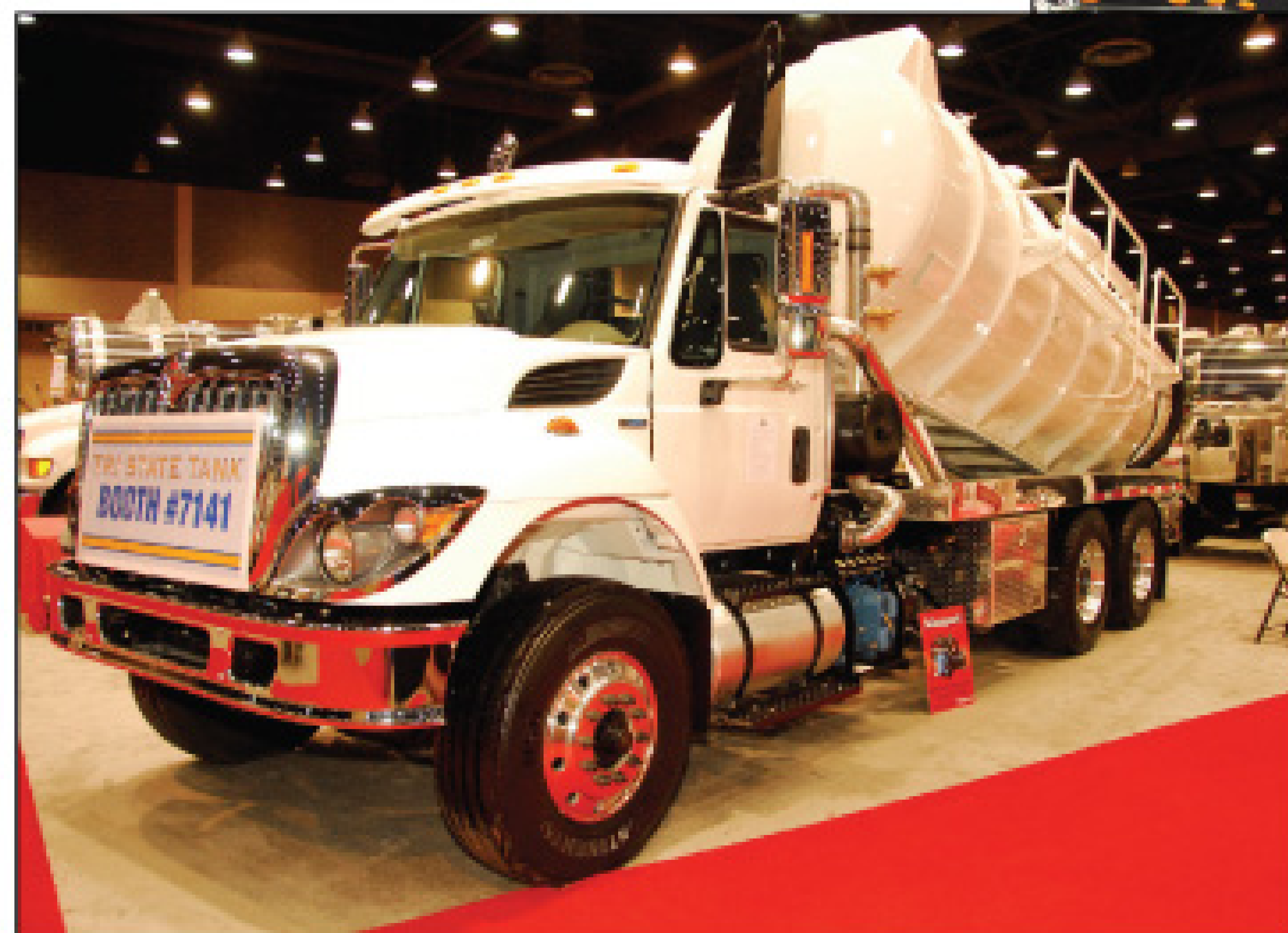
Among the trucks featured at the 2009 Expo were a 2009 International (above) built by Best Enterprises Inc. for A & G Pumping of King City, Calif., and this International 7500 (left) built by Tri State Tank with 3,800-gallon aluminum tank painted white.
