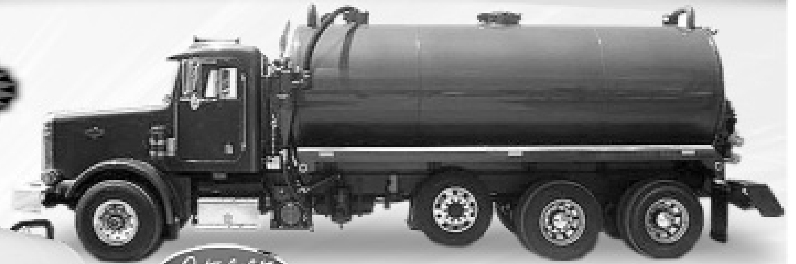
2001 PETERBILT 357 Mileage Less Than 180K, 357 CAT Power, 8 LL Transmission, Heavy Duty Suspension, 46K Rear - 21K Fronts, 4800 Carbon Steel Tank
