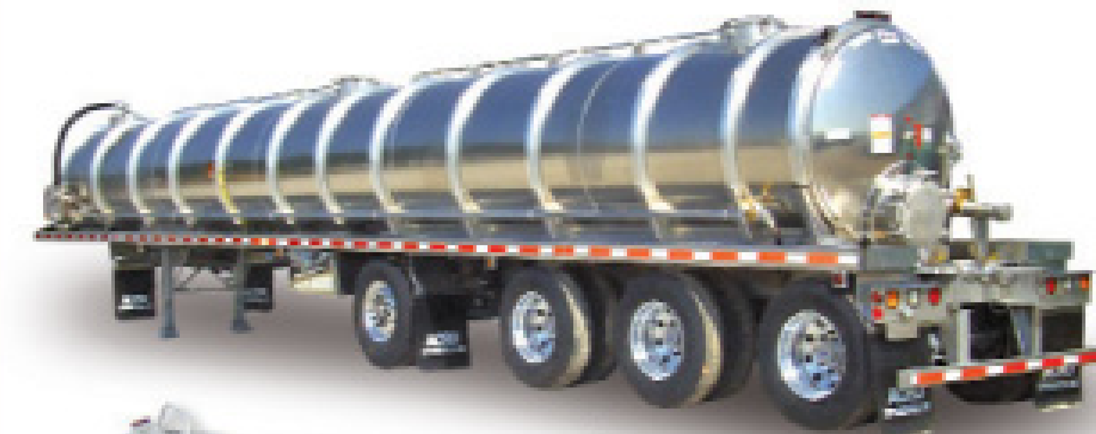
7,150-GALLON ALUMINUM DOT-412 VACUUM DUMPER
