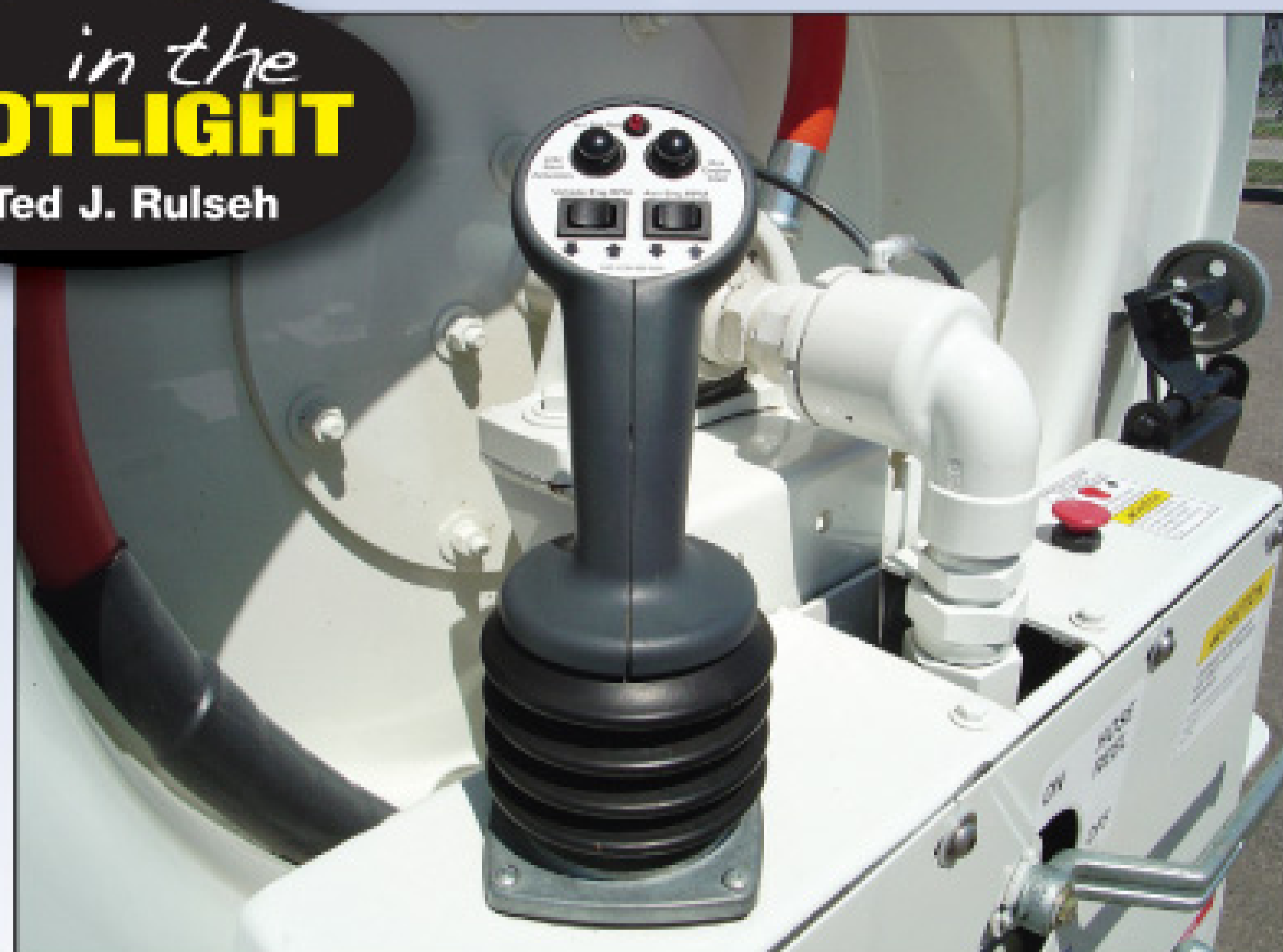
The joystick controller for Vac-Con and Xcavator machines provides added convenience in the operation and maintenance of hardworking rigs.
