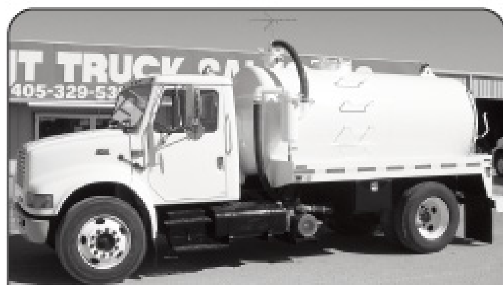
2000 IH 4700, DT466E, 5-spd., non-CDL, double frame, new Wally 403HR vacuum pump, new 1600 gallon vacuum tank.
