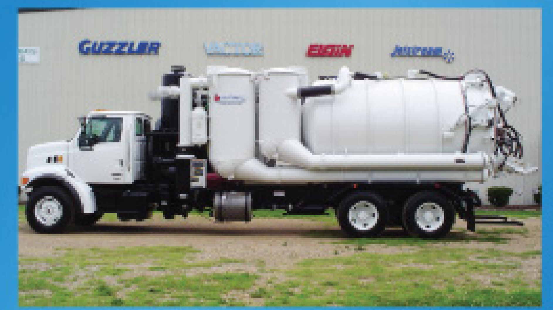
Unit #06873 Sterling LT9501 Hibon 8702 27" Blower, Dense Phase Offload System, Auto. Transmission READY TO WORK!
