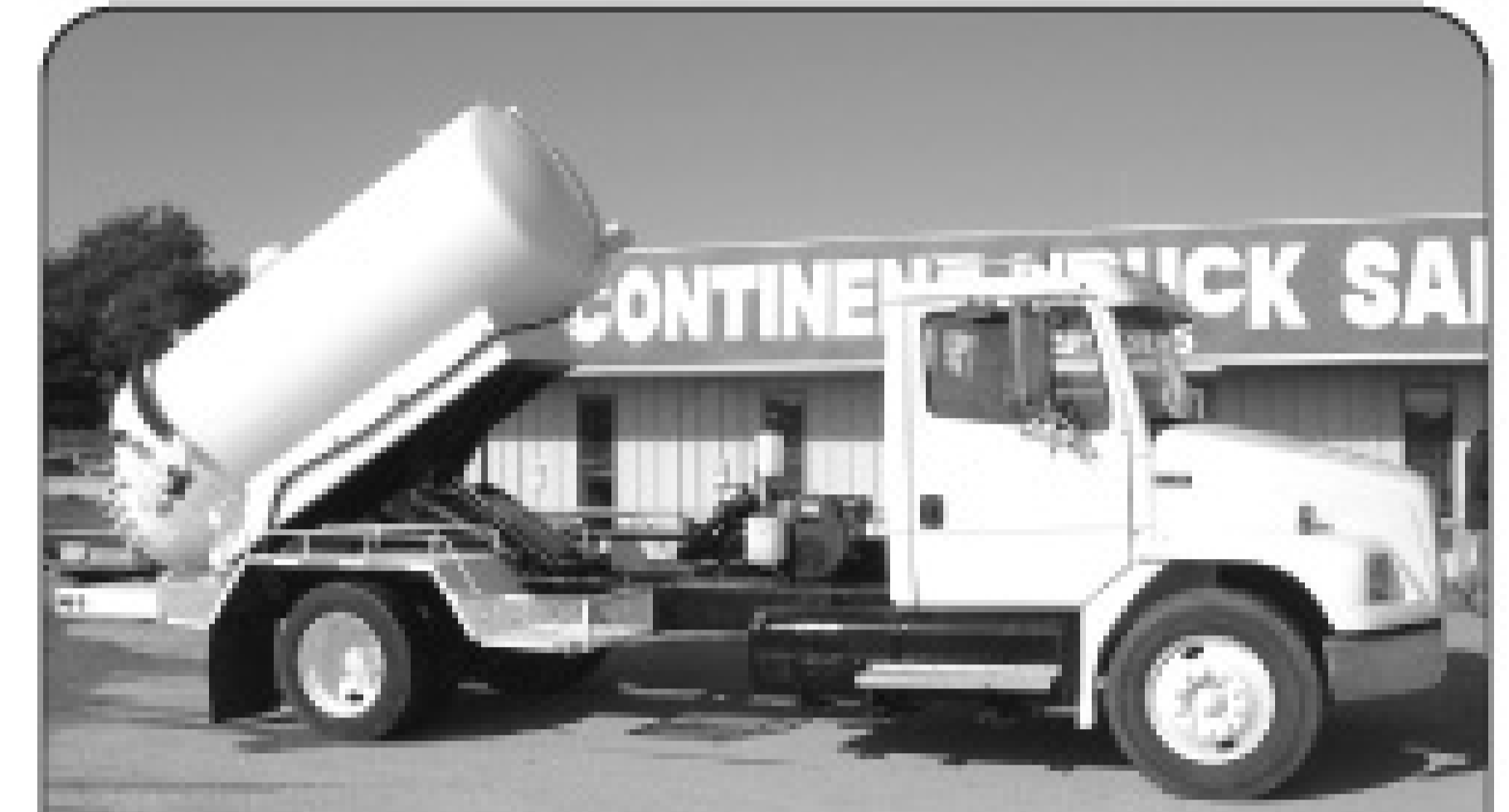
1998 Freightliner FL60, Cummins 5.9 (210 hp), 6-spd., Masport H75V vacuum pump, General 47 series triplex, 1100/200 gallon vacuum tank.
