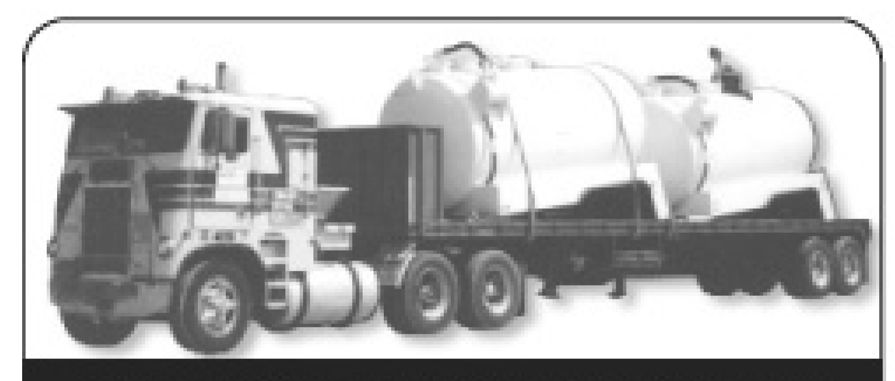
1989 Chevrolet C70, 8.2 ltr. diesel, 5+2 air brakes, double frame, MEC 5000 vacuum pump, 1500 gallon vacuum tank.
