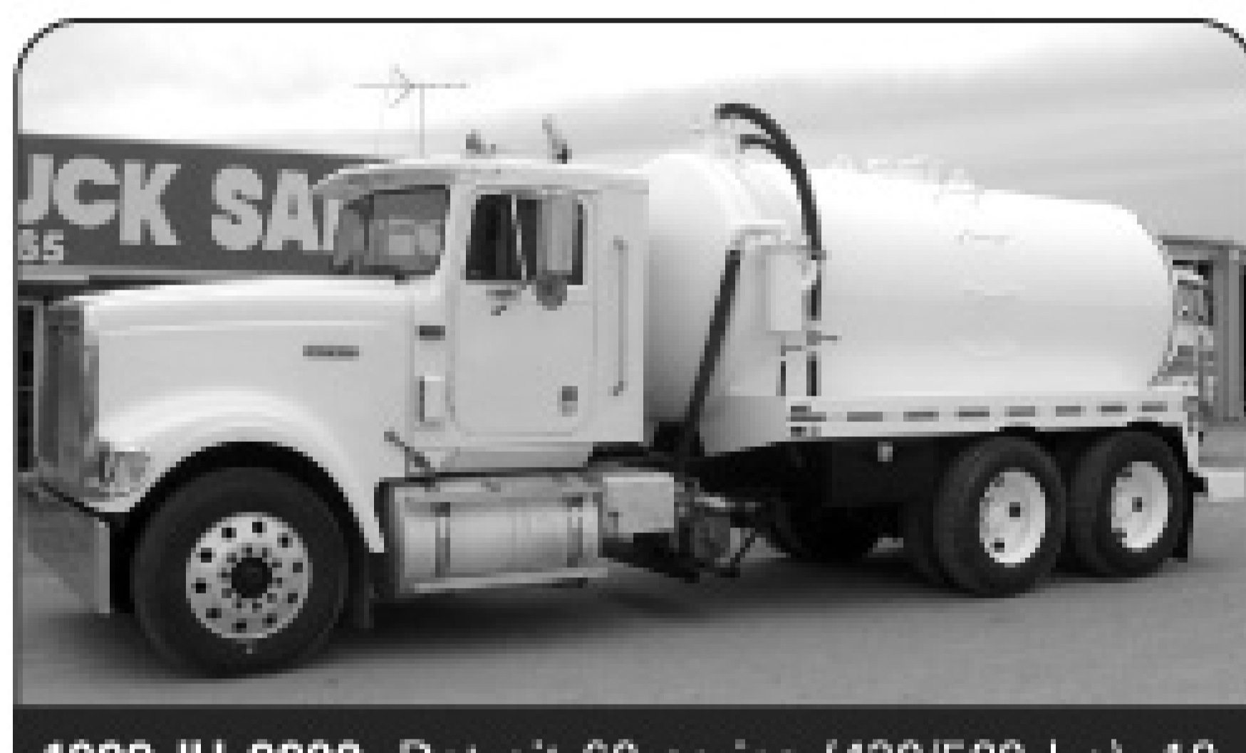
1999 IH 9900, Detroit 60 series (430/500 hp), 10-spd., new Wally 753LN vacuum pump, new 3000 gallon vacuum tank.
