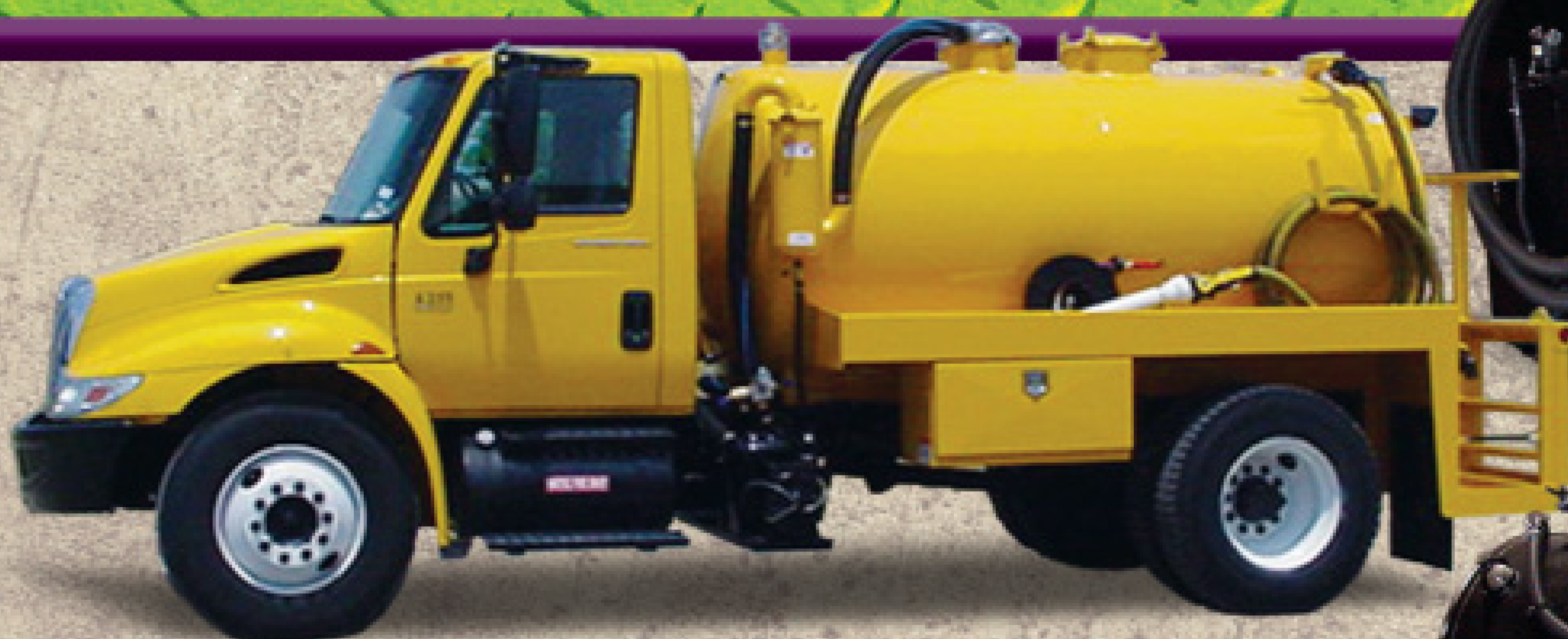
1550 Gallon Steel Portable Toilet Unit 1100 Waste & 450 Fresh Water
