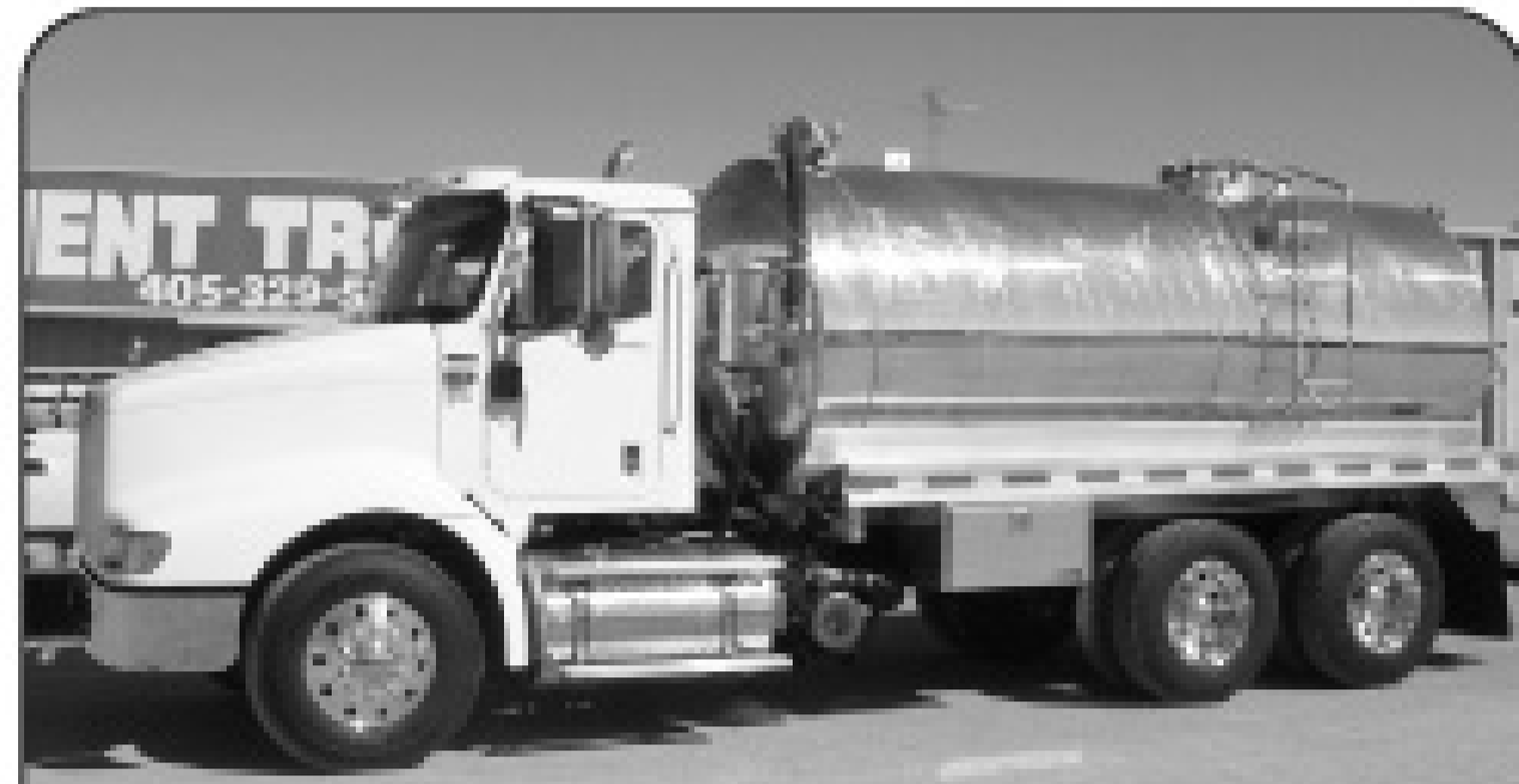
2003 IH 9100I, Cummins N14 (435 hp), 10-speed, double frame, new Wally 753LNHR vacuum pump, new 3800 gallon aluminum vacuum tank.
