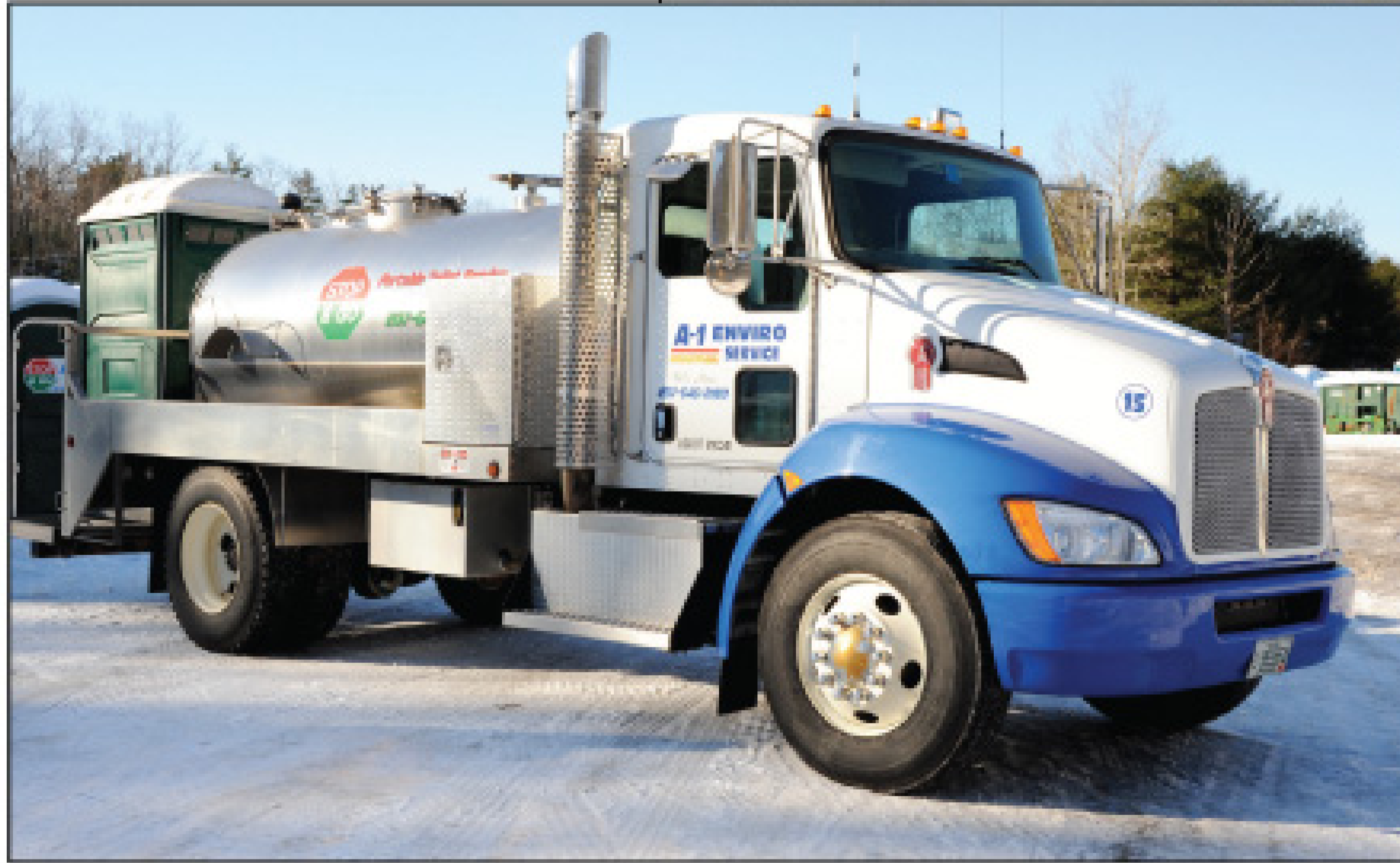
Above: A-1’s T800 Kenworth roll-off truck, equipped with a 75,000-pound hoist, loads a 15-yard container. At left: A Kenworth T270 service truck with 1,500-gallon stainless steel tank by Best Enterprises and Masport pump transports a PolyJohn PJ3 restroom.
