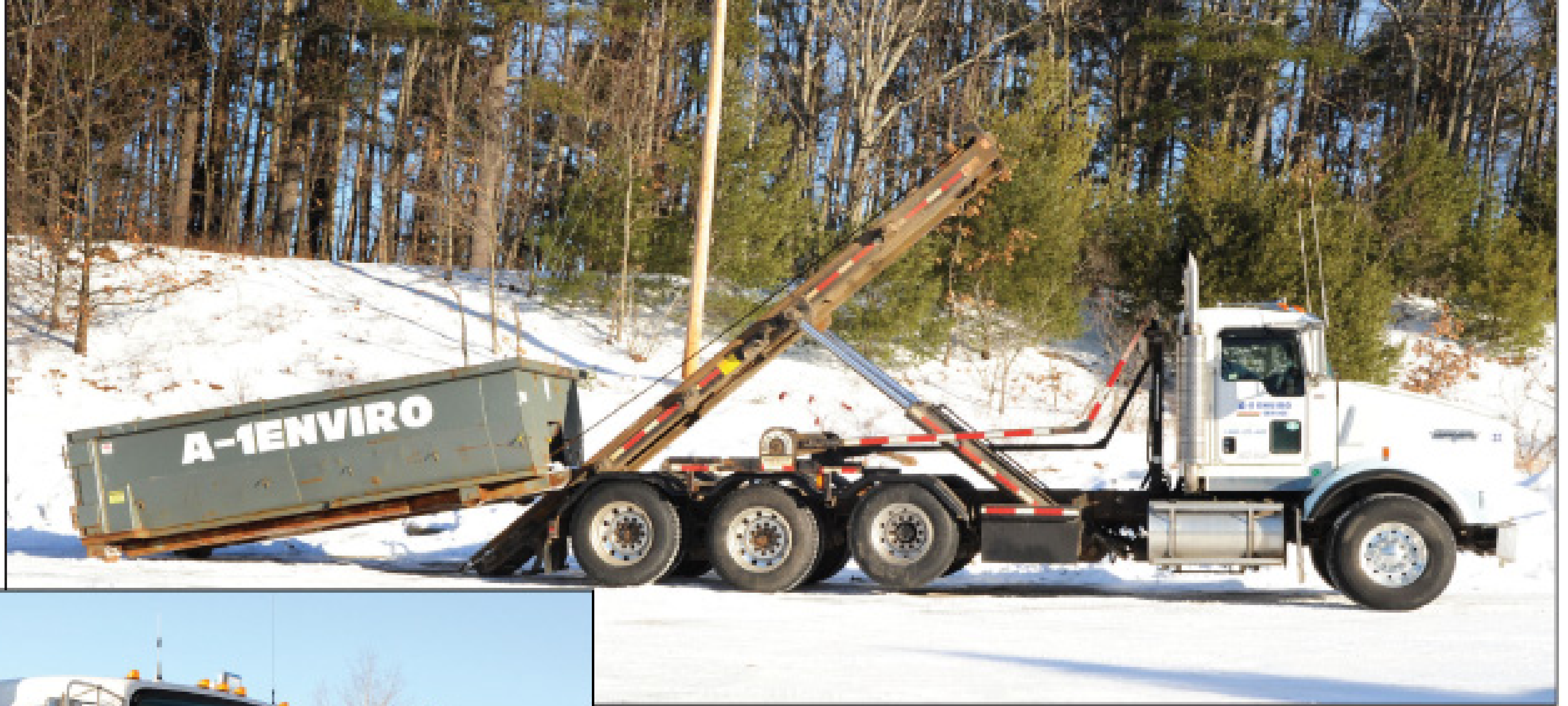
Above: A-1’s T800 Kenworth roll-off truck, equipped with a 75,000-pound hoist, loads a 15-yard container. At left: A Kenworth T270 service truck with 1,500-gallon stainless steel tank by Best Enterprises and Masport pump transports a PolyJohn PJ3 restroom.
