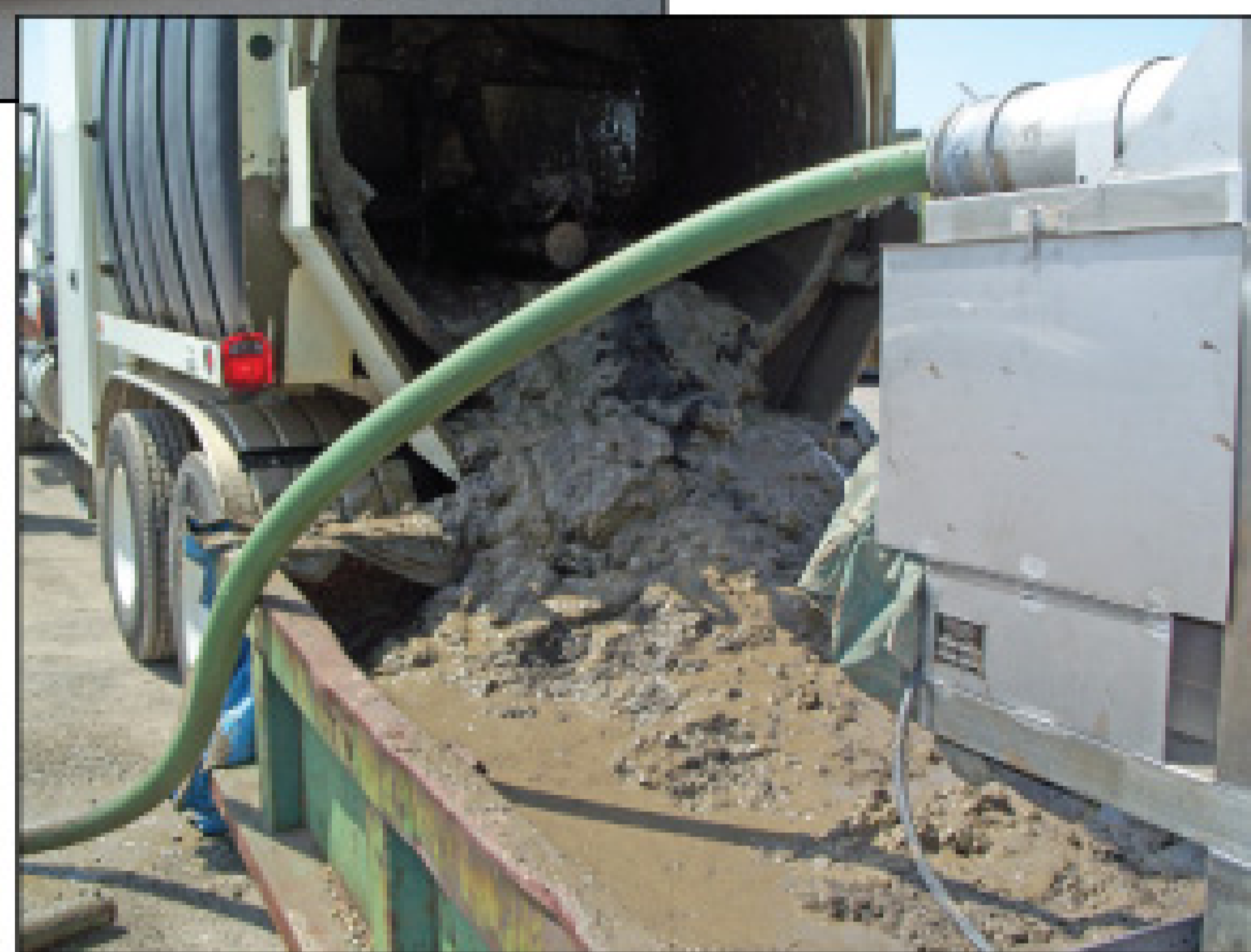
The IFRS 36 has a compact design to fit in many locations (above). The unit is hydraulically powered and can run off a truck's hydraulic system.
