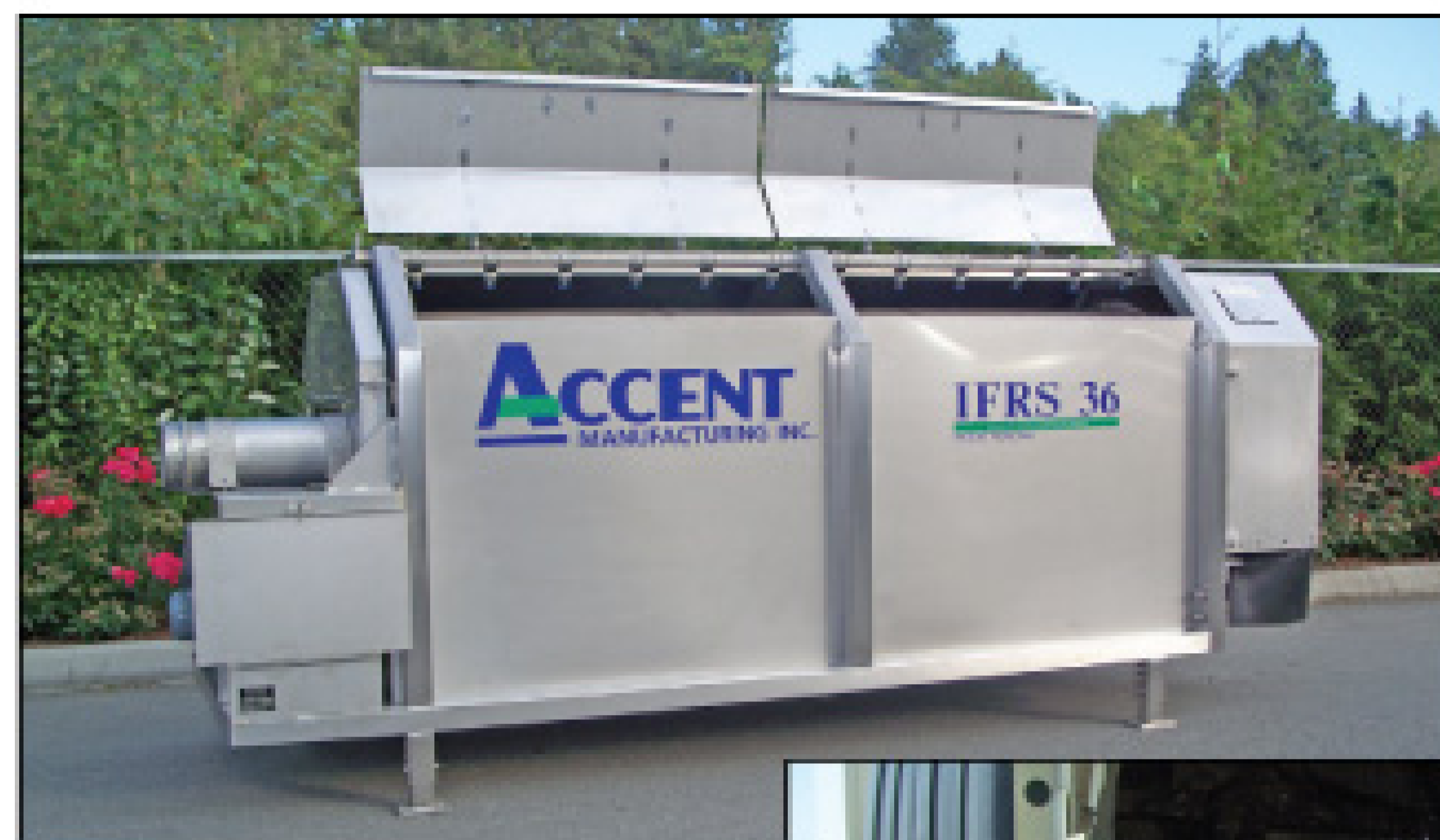
The IFRS 36 has a compact design to fit in many locations (above). The unit is hydraulically powered and can run off a truck's hydraulic system.
