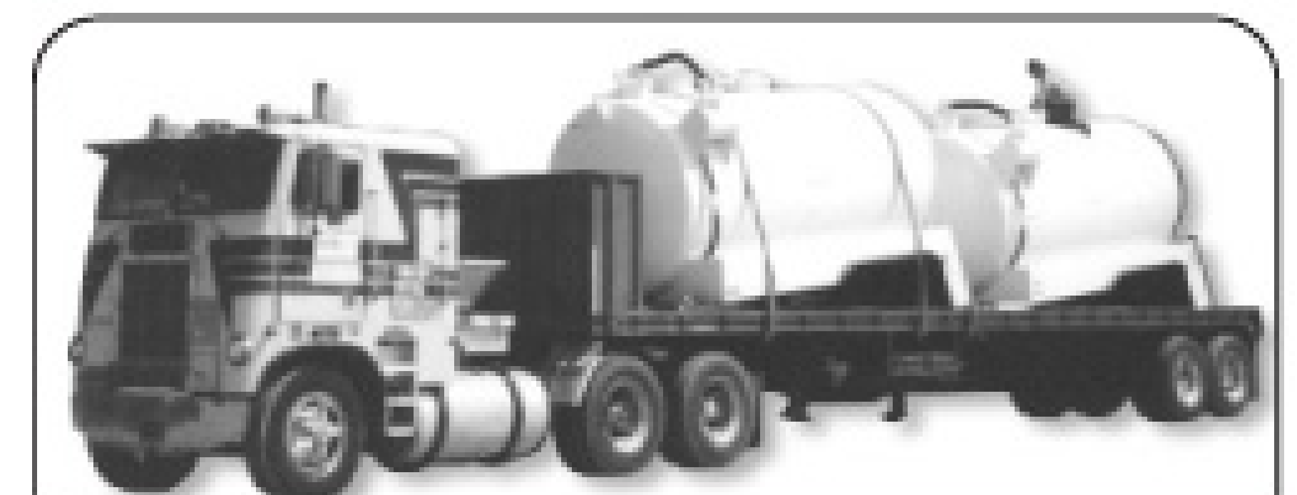
1989 Chevrolet C70, 8.2 ltr. diesel, 5+2 air brakes, double frame, MEC 5000 vacuum pump, 1500 gallon vacuum tank.
