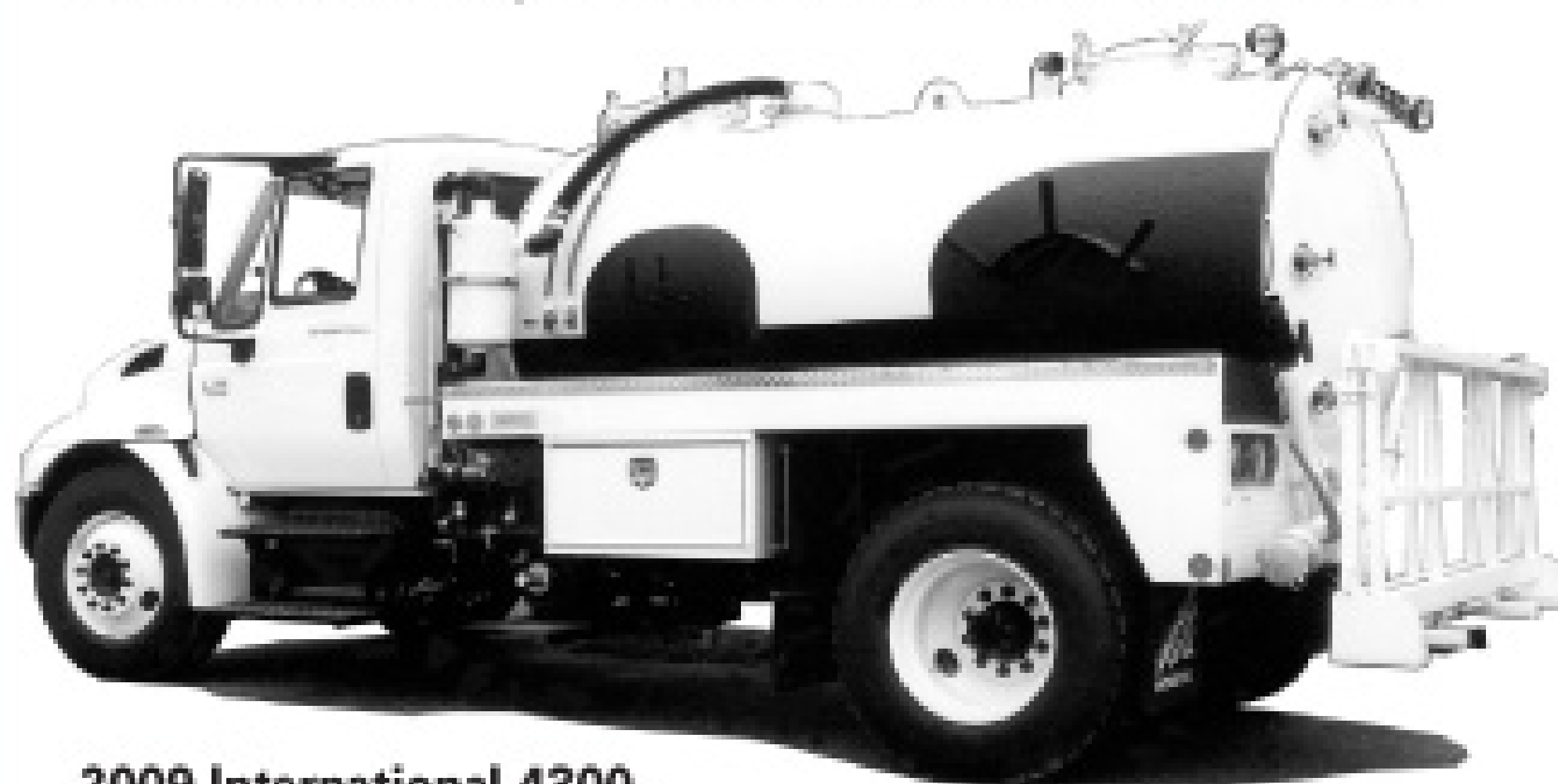
2009 International 4300, 220 hp DT466, Allison auto. trans., air brakes, 25,999 GVW, air conditioned, total tank capacity: 1100 waste/400 fresh, Masport HXL75V pump. IMMEDIATE DELIVERY! Also, 1500 gal. tanks READY FOR IMMEDIATE DELIVERY.
