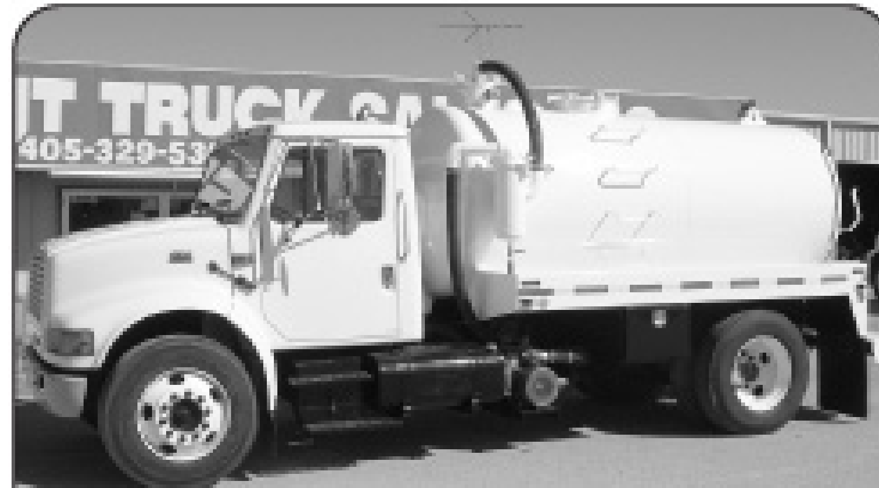
2000 IH 4700, DT466E, 5-spd., non-CDL, double frame, new Wally 403HR vacuum pump, new 1600 gallon vacuum tank.
