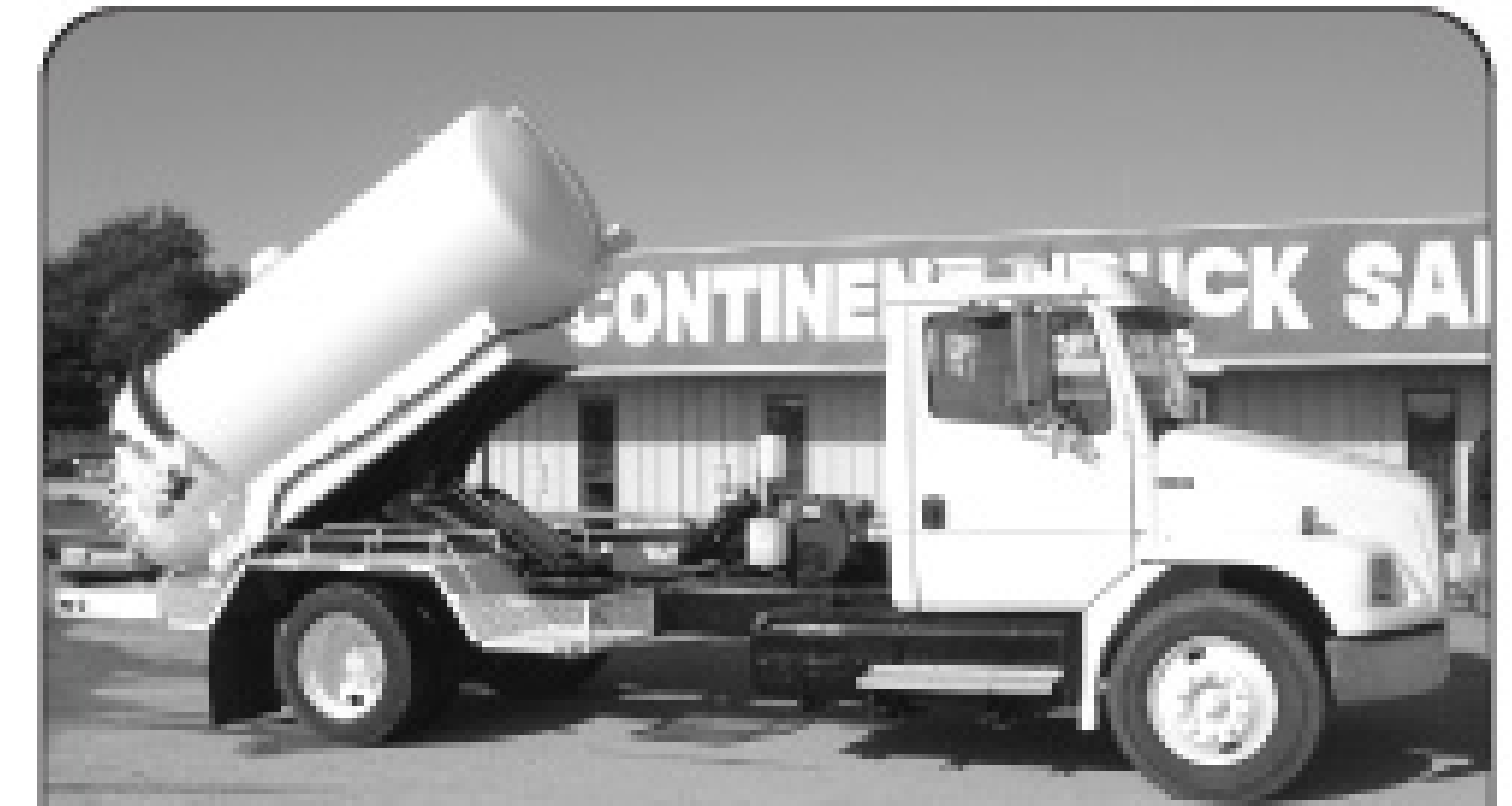
1998 Freightliner FL60, Cummins 5.9 (210 hp), 6-spd., Masport H75V vacuum pump, General 47 series triplex, 1100/200 gallon vacuum tank.
