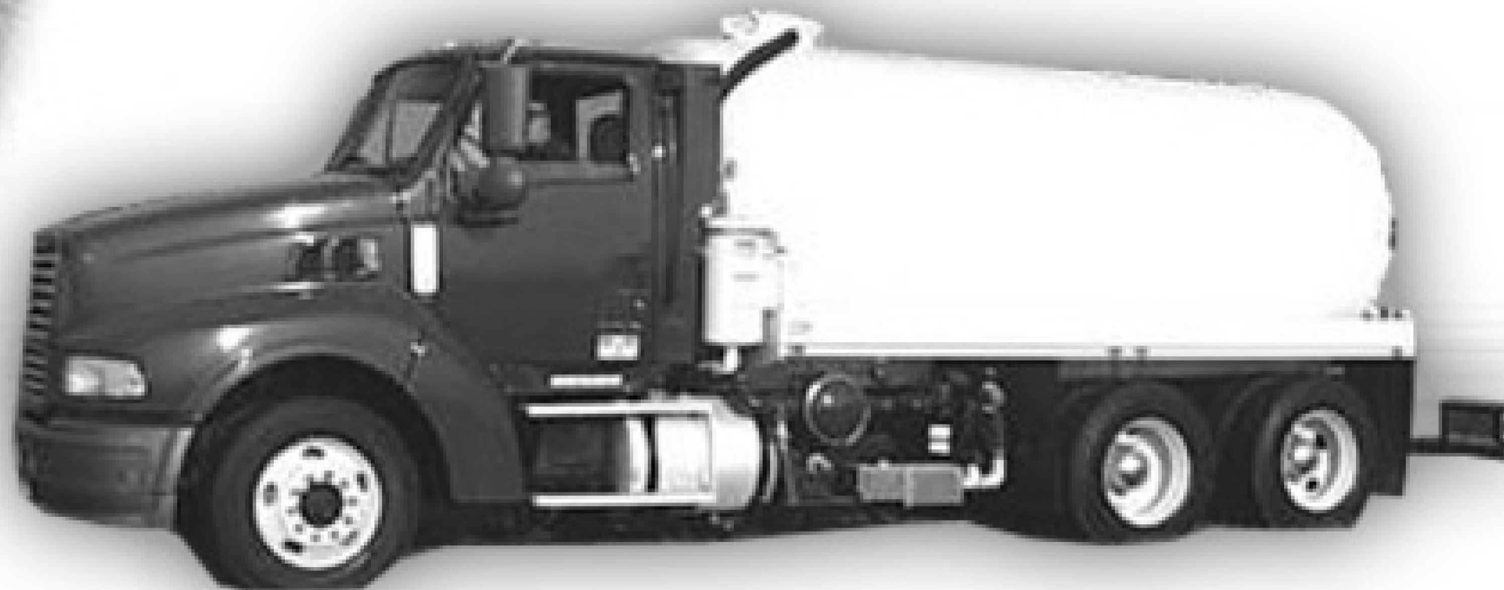
Advanced Plumbing Technologies, Olympia, WA 1999 Sterling w/ 3250 gallon vac/pres tank
