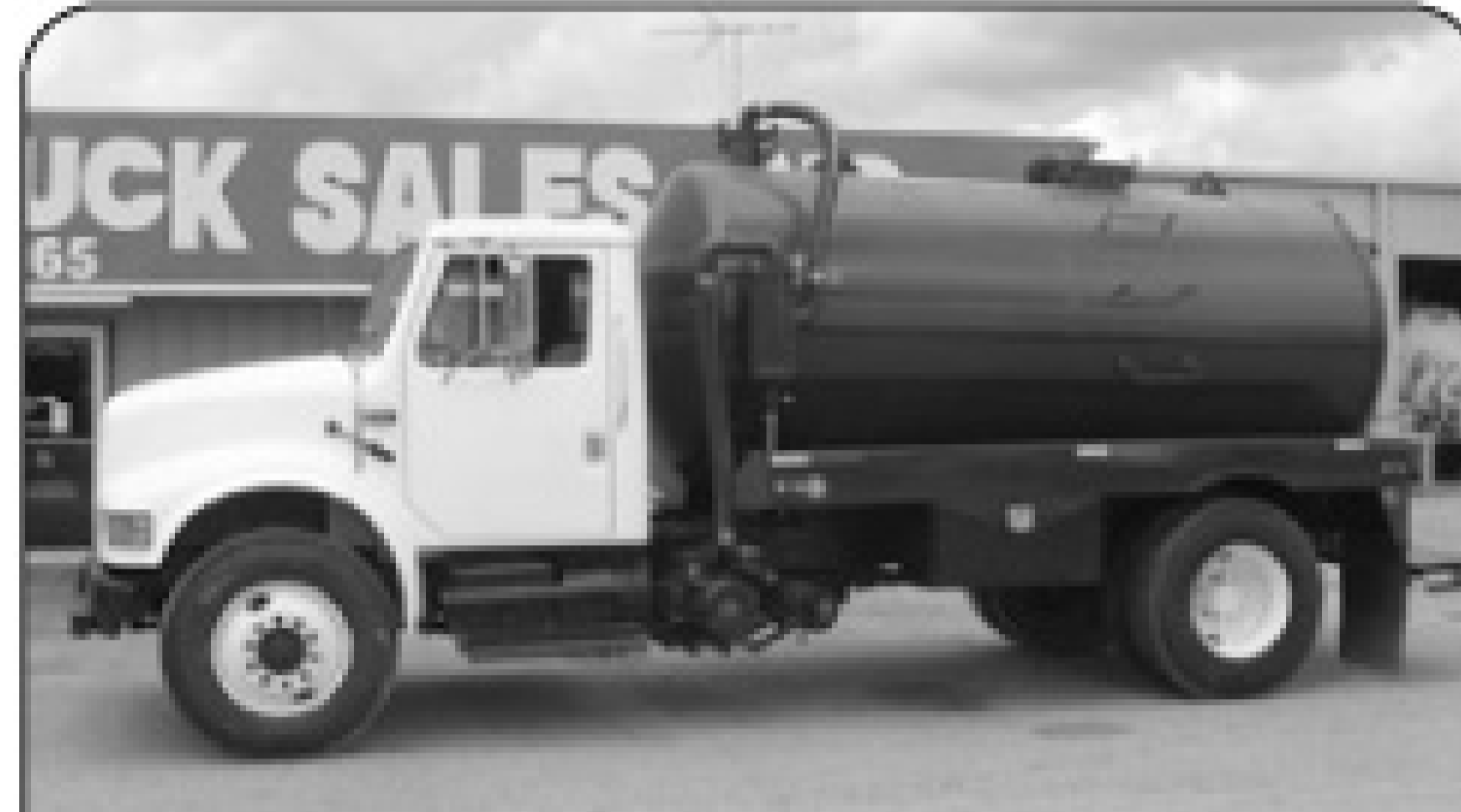
1992 IH 4900, DT466, 6-spd., 33K GVW, double frame, Wally 553HR vacuum pump, 2300 gallon vacuum tank.
