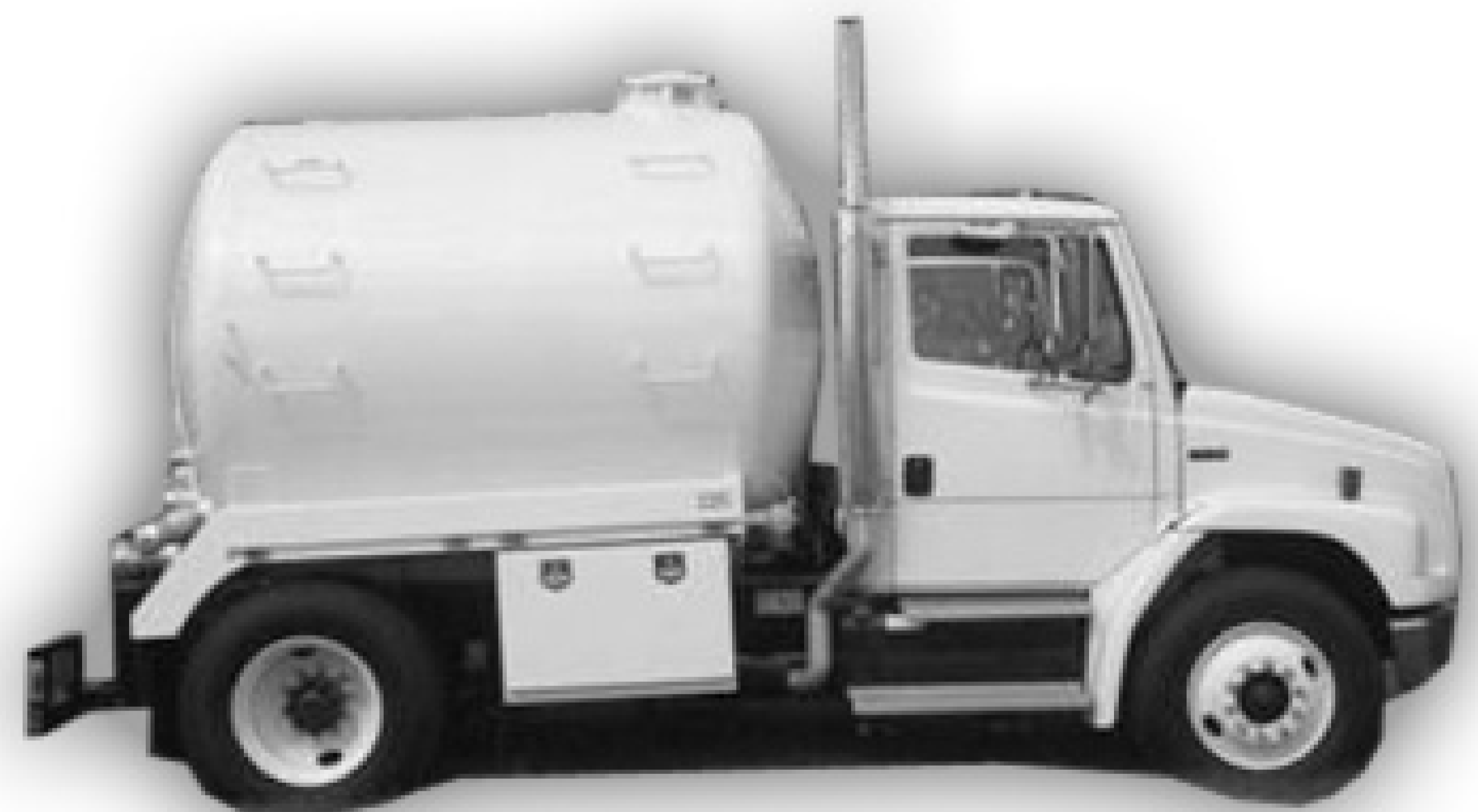
Unitek Environmental, Barrigada, Guam 2000 Freightliner w/2000 gallon vac/pres tank
