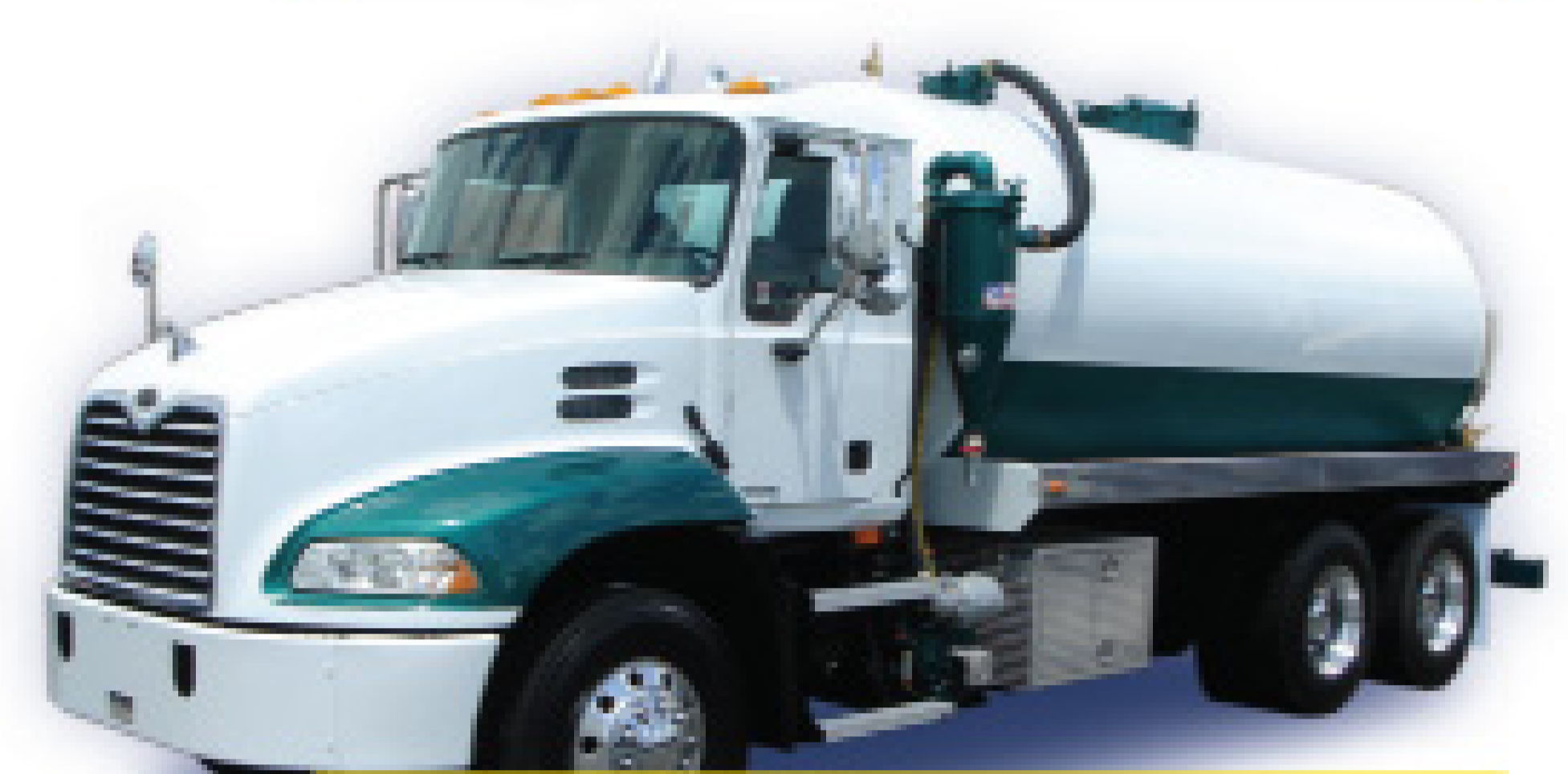
2005 MACK VISION 4000 Gal US Tank, Double Frame, Jurup LC 420 Water Cooled
