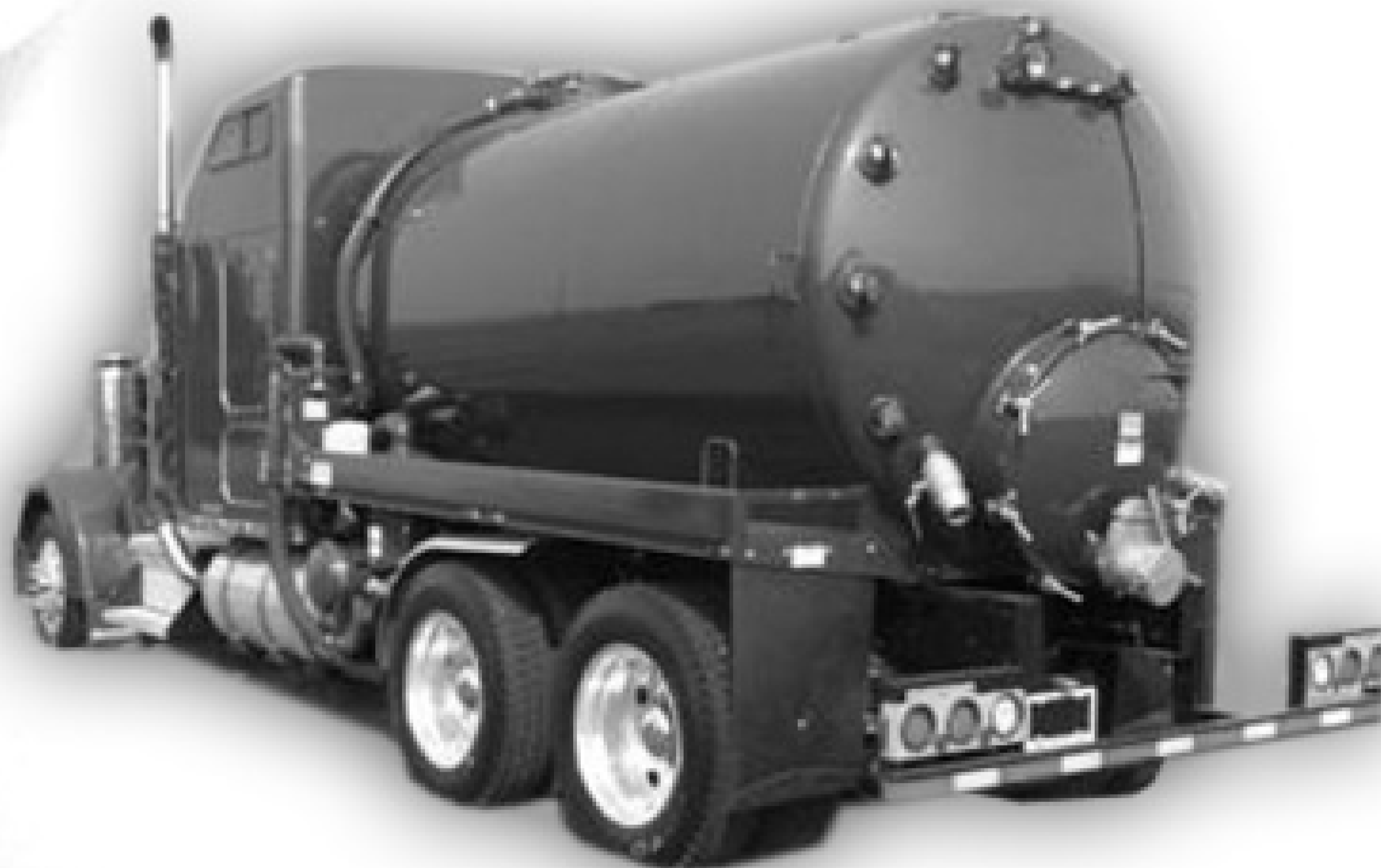
S & K Transport, Darby, MT 3000 gal. vac/pressure tank w/Masport HXL15V
