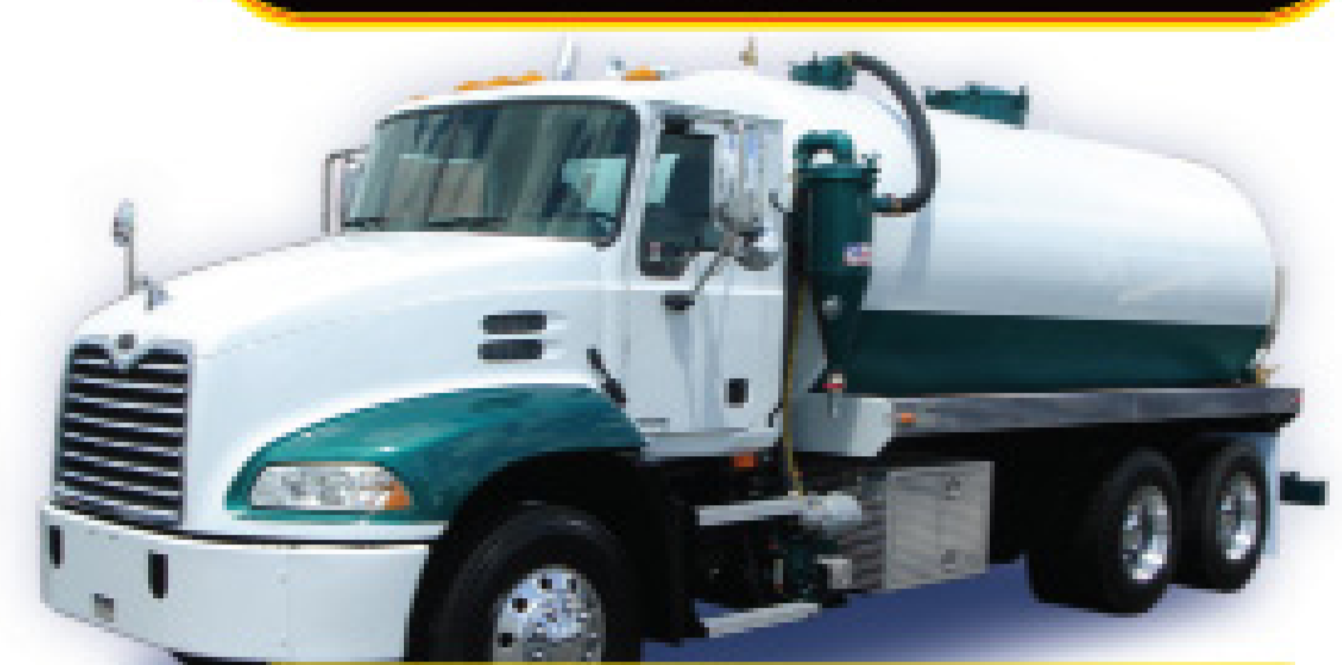
2005 MACK VISION 4000 Gal US Tanks, Double Frame, Jurup LC 420 Water Cooled
