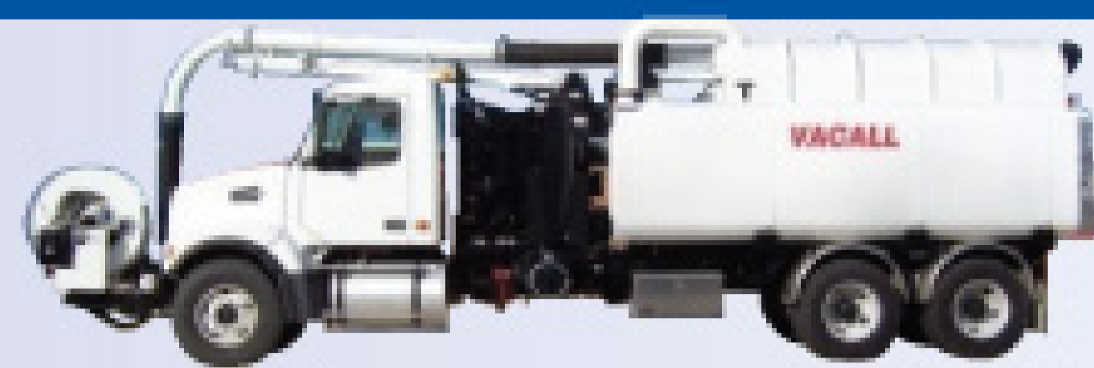
New 2007 Volvo VHD 64F, VacAll 1215 Combination Sewer Cleaner, Available with Hydro-Excavation package, Hibon TS56 Blower 18 Hg, MSS 55 Water pump 80 gpm @ 2000 psi
