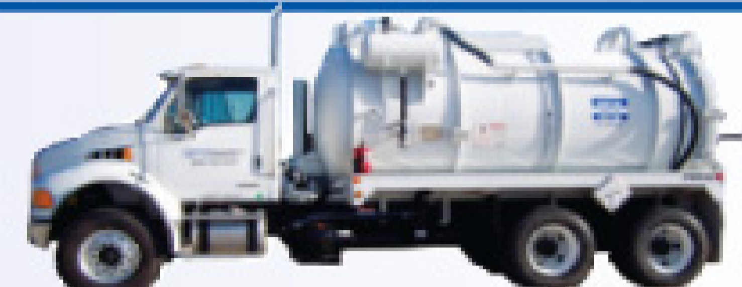
Coming soon; new 2008 Sterling Acterra, Presvac DOT 407/412 dump type vacuum unit with choice of PV750 vacuum pump or VTB 820 blower.
