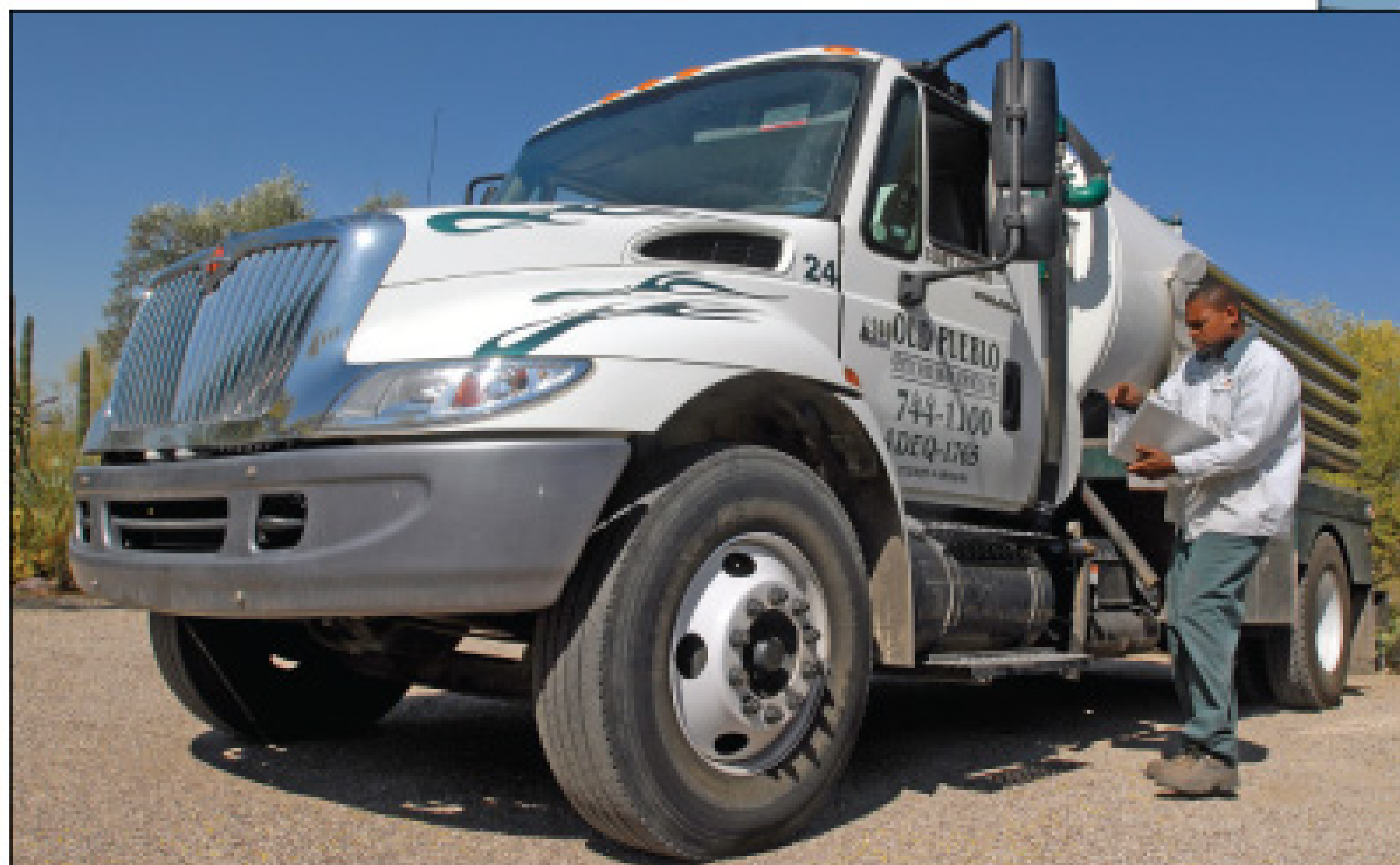
Service technician Zep Homes stands next to an International 4300 with 2,500-gallon tank. Old Pueblo Septic and Drain Service has seven vacuum trucks in its fleet.
