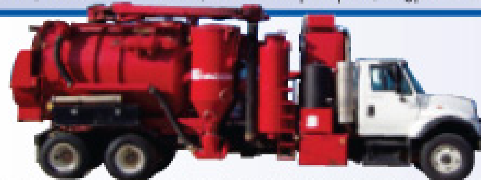
2005 International 7600, Vac-con 4716SMXD Hydro-Excavator, 16 cy Debris tank, 3000 psi @ 15 gpm cat 3560 73,370 miles, 2560 engine hr. 1175 blower hr. 1021 DVJ
