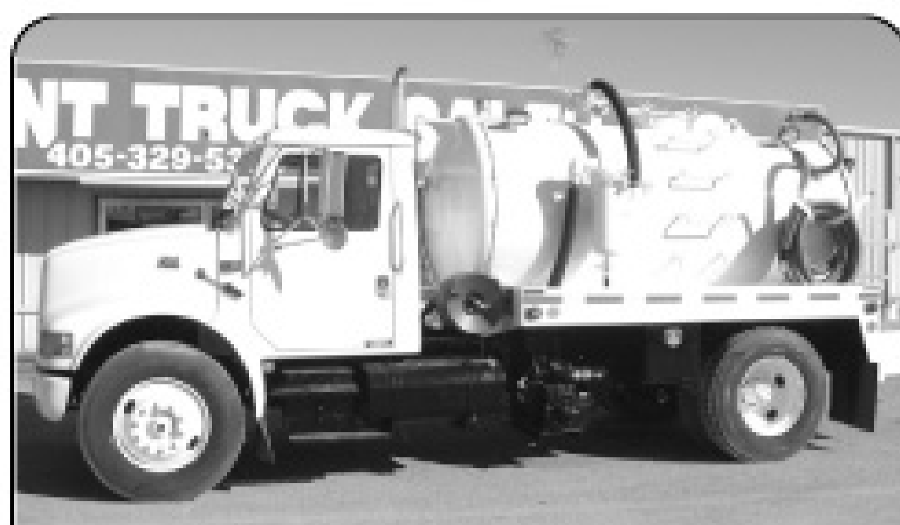
2001 IH 4700, DT466E, Allison auto, non-CDL, air brakes, new MEC 6500 vacuum pump, new 1100/400 vacuum tank.
