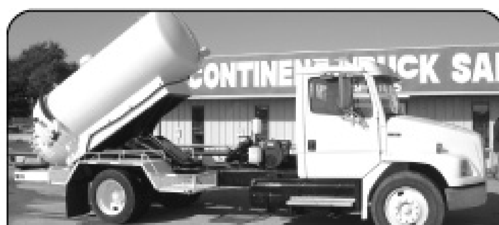
1998 Freightliner FL60, Cummins 5.9 (210 hp), 6-spd., Masport H75V vacuum pump, General 47 series triplex, 1100/200 gallon vacuum tank.
