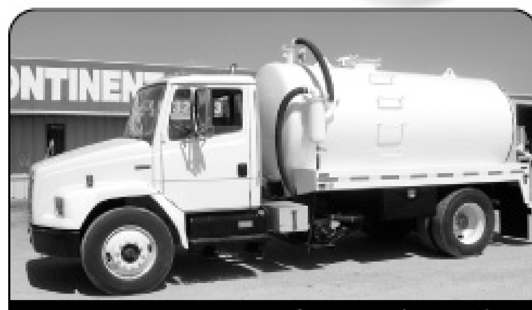
2001 Freightliner FL70, Cat 3126 (230 hp), 6-speed, 33,000 lbs., double frame, new MEC8000/PAL vac pump, new 2300 gallon vacuum tank.
