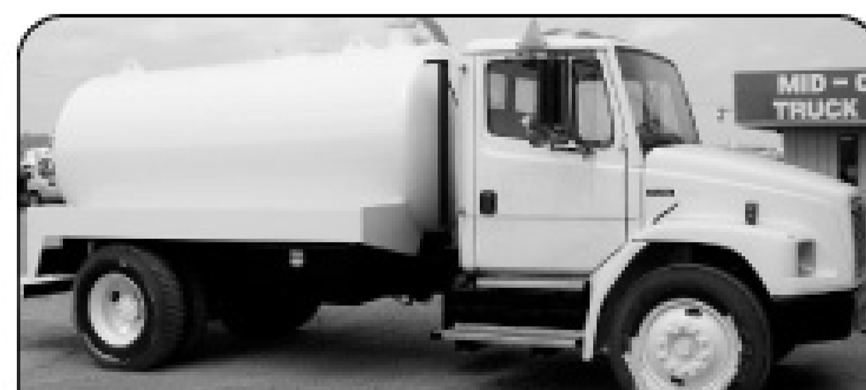
2001 Freightliner FL70, Cat 3126 (190 hp), 5-speed, non-CDL, new Masport HXL75V vac pump, new 1600 gallon vacuum tank.
