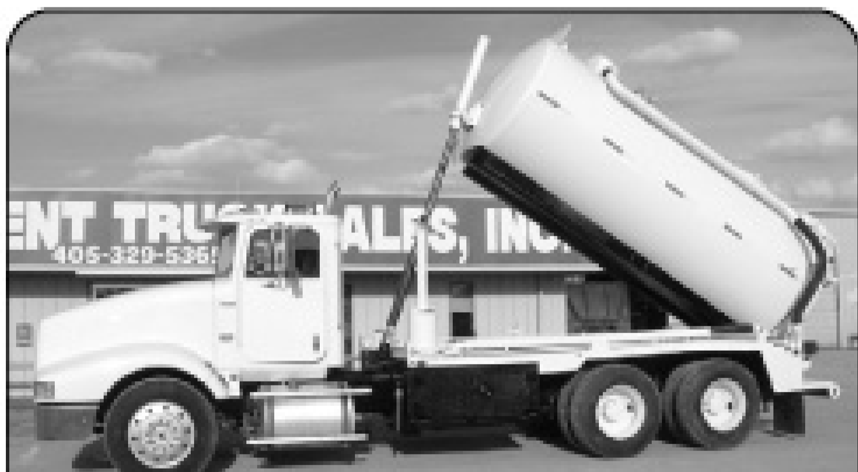
1990 IH 9400, Cummins NTC350 w/fresh inframe, 9-spd., new Wally 753LNHR vac pump, 3500 gallon vacuum tank w/full opening rear door.
