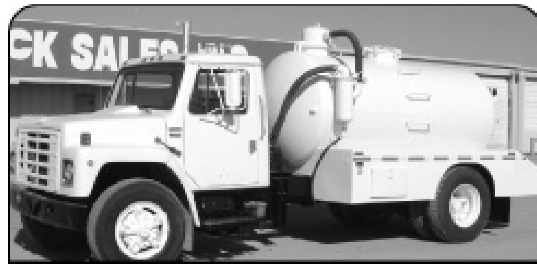
1981 IH S1854, DT466, 10-speed, Wally 403 HR vac pump, 1600 gallon vacuum tank.
