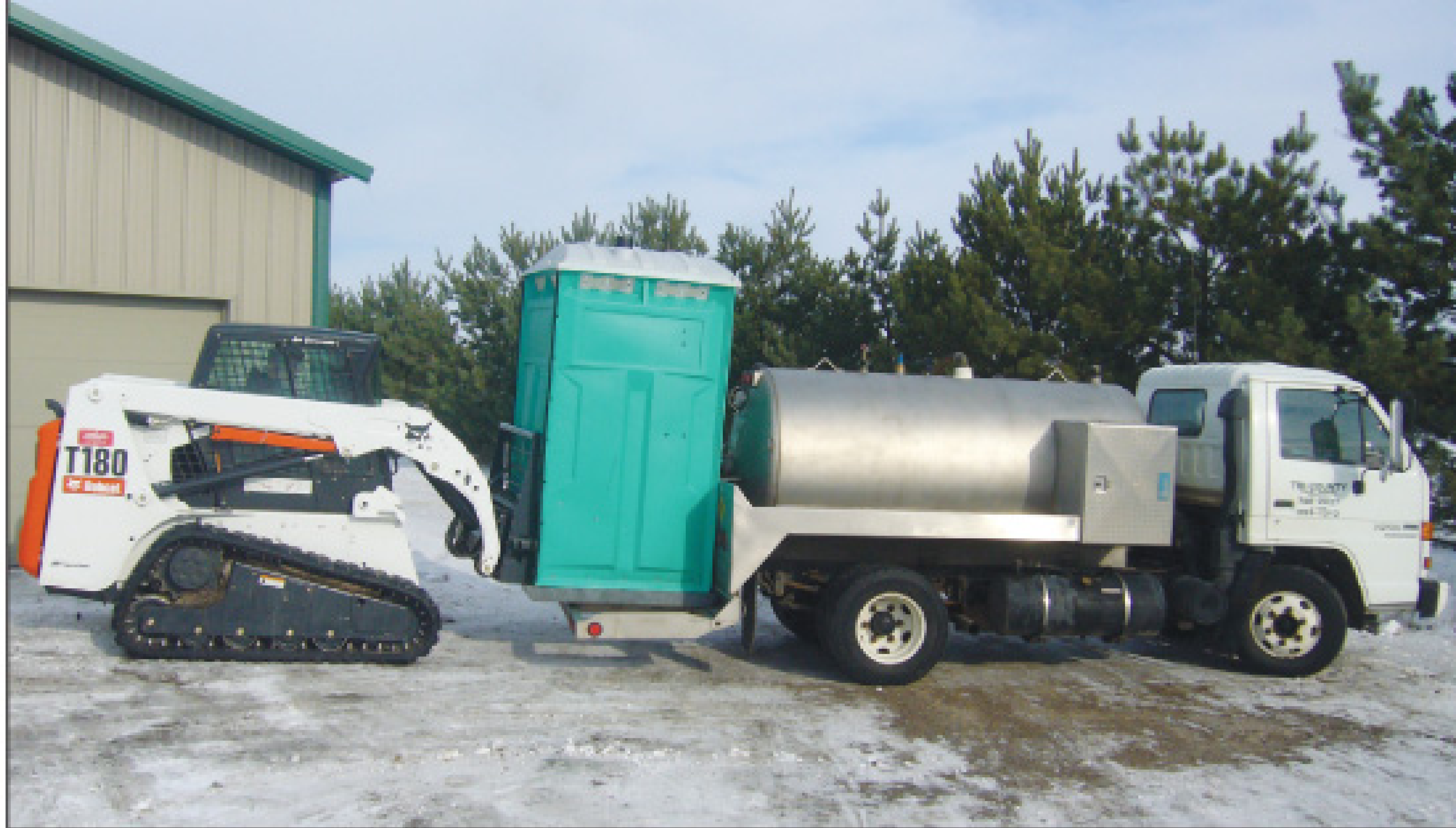
Forks are added to a Bobcat T-180 to load a Satellite Industries Tufway restroom to the back of Tri-County's portable sanitation truck, a 1995 Isuzu with an 800-gallon stainless-steel tank.
