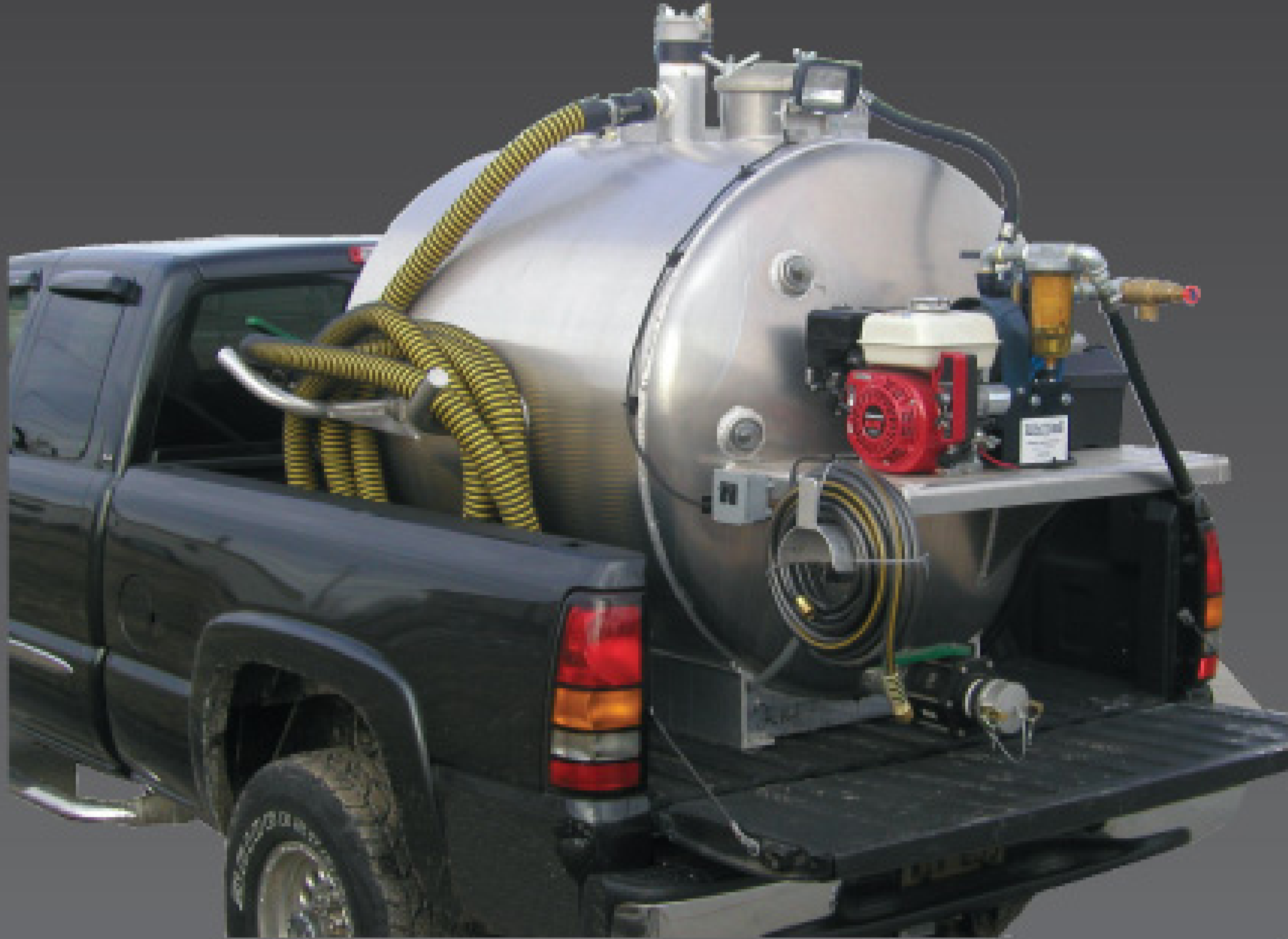
Masport H1V or Conde Super 6 vacuum pump w/ 4-way valve
