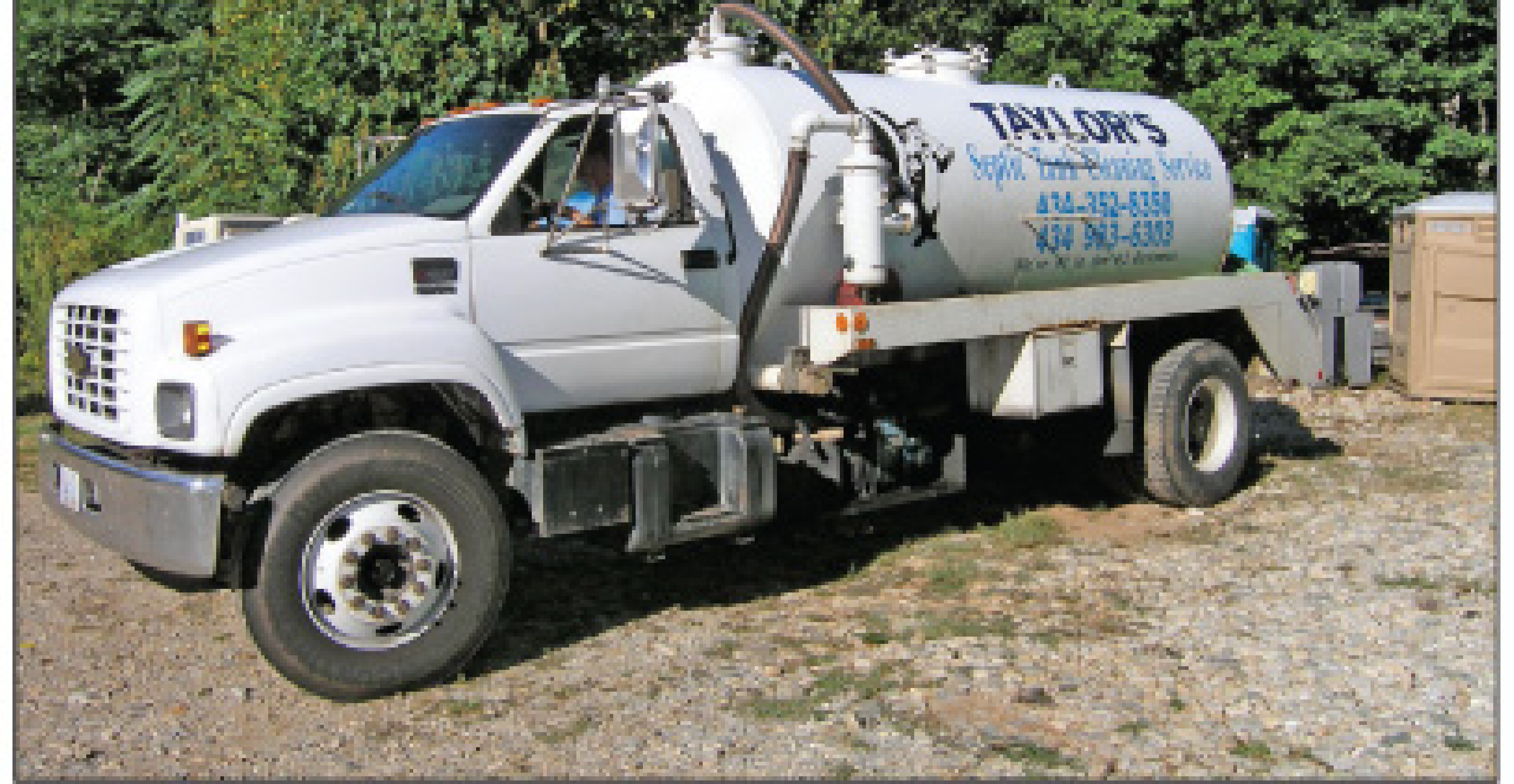
A 1997 Chevrolet C7500 service truck with a 2,500-gallon steel tank is a staple among three pumper trucks used mainly for residential septic service.
