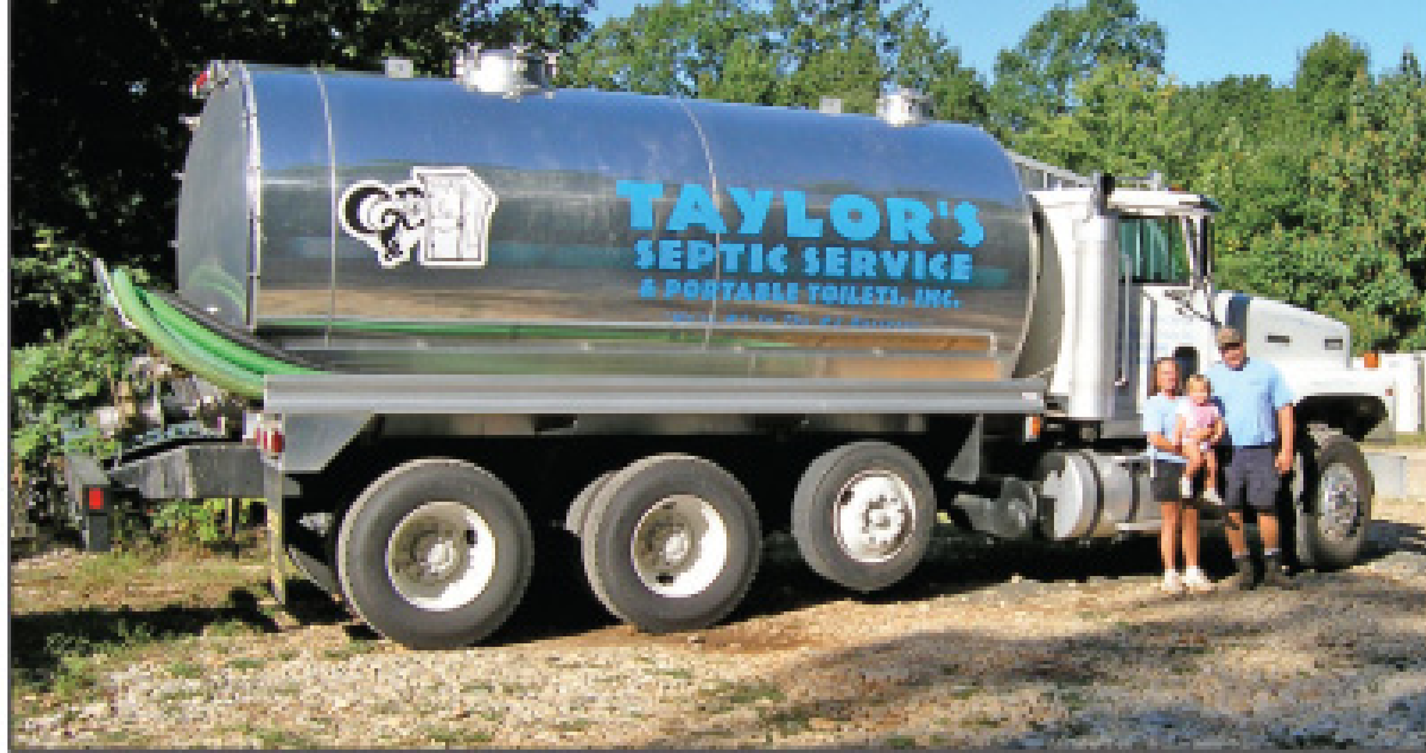
John and Penny Taylor, with granddaughter Madisyn, show off their 1999 International vacuum truck with 4,500-gallon aluminum tank from Amthor International.
