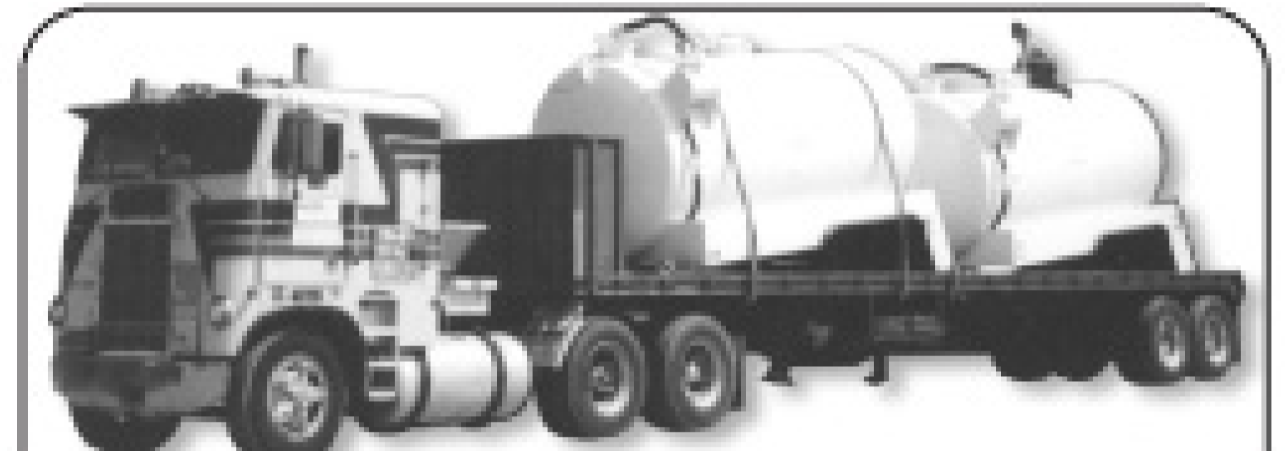
2004 Kenworth T300, Cat C7 (210 hp), 6-spd., 33K GVW, new Wally 753HR (350 cfm), new 2600 gal. aluminum vacuum tank, 2-yr. nationwide drivetrain warranty.
