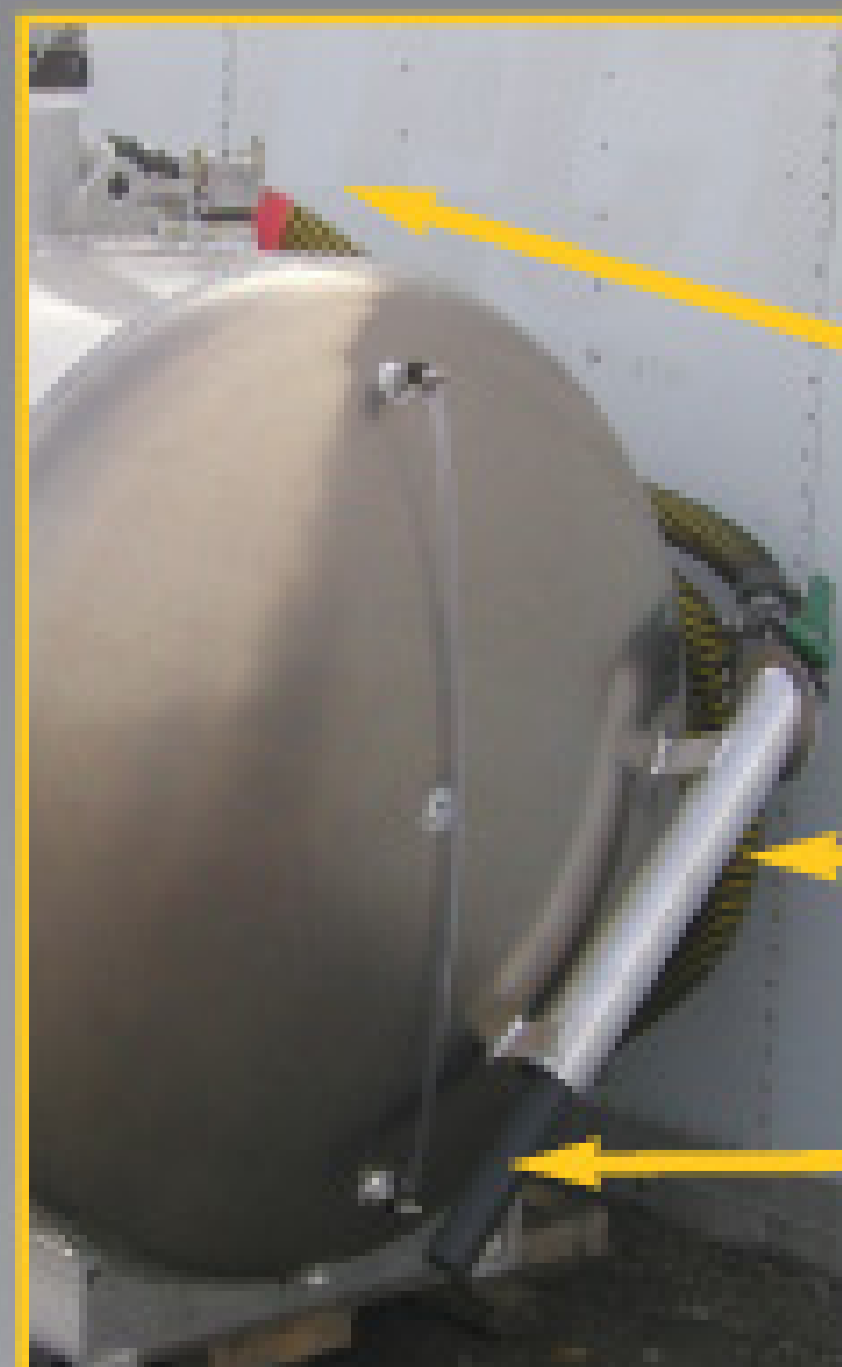
3" valve on discharge with adapter and dust cap
