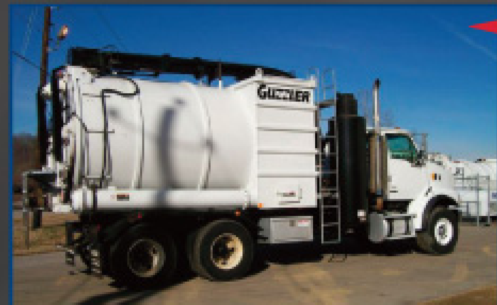
ID #85085, 2005 Guzzler CL, 1024 16" Vacuum, Hydraulic boom and vibrator READY TO WORK!
