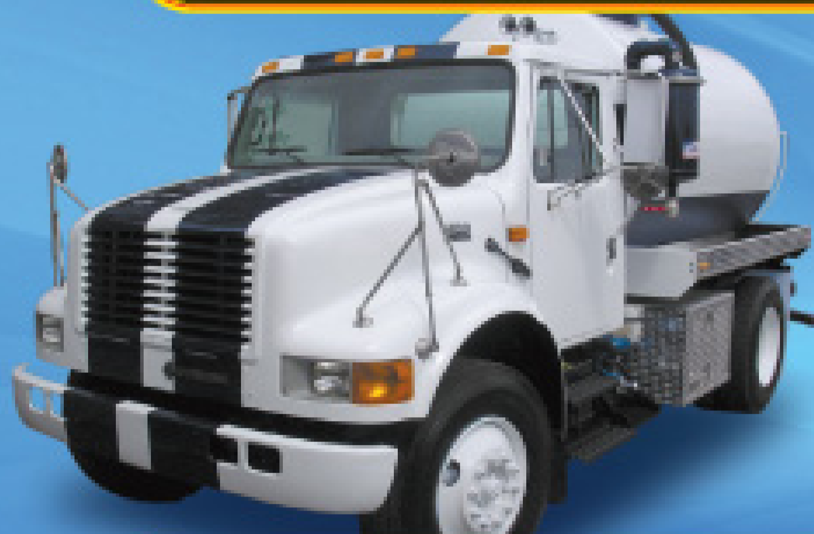
2000 INTERNATIONAL 4900 2200 gal US Tanks, Double Frame, MASPORT HLX75
