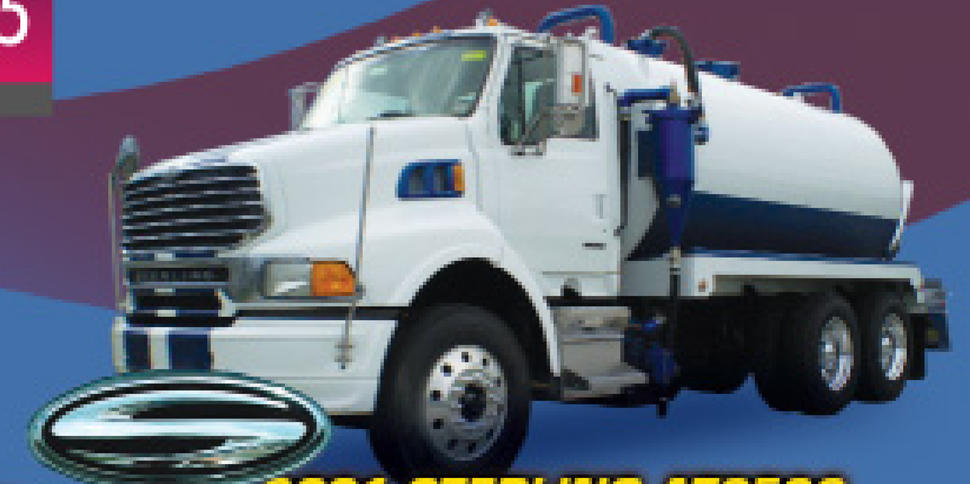
2001 STERLING AT9522 4000 Gallon Carbon Steel Tank, Fruitland Pump RCF 500 350 C.F.M.
