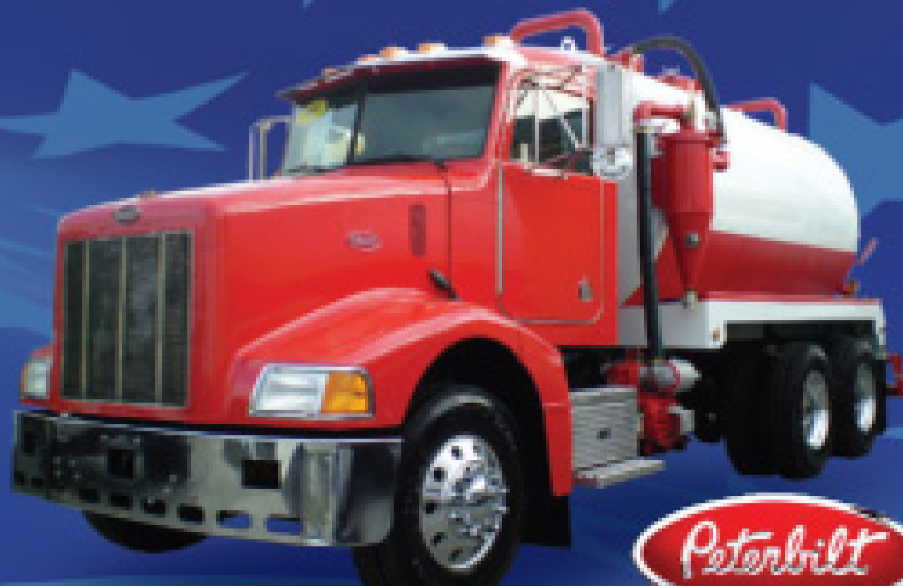
1999 PETERBILT C12 Cat, 10 Spd., 430 HP, 3600 Gallon Carbon Steel Tank, Jurop Pump LC 420 Contender (Extras Included) Available for the Pumper Show.
