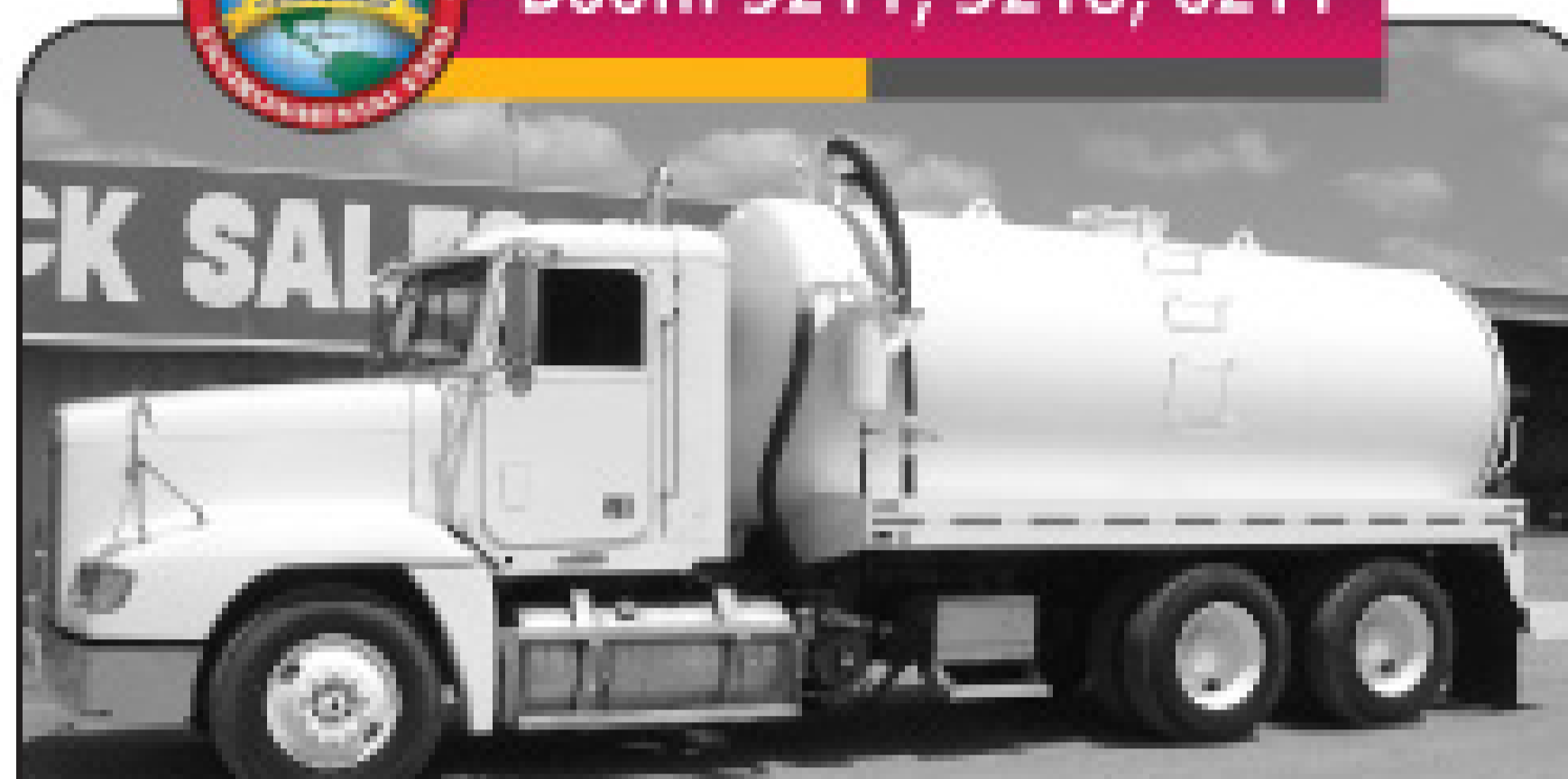
2000 Freightliner, Detroit 60 series (430/470 hp) w/fresh overhaul, 10-speed, double frame, new Wally 753LNHR vac pump, new 3400 gallon vacuum tank.
