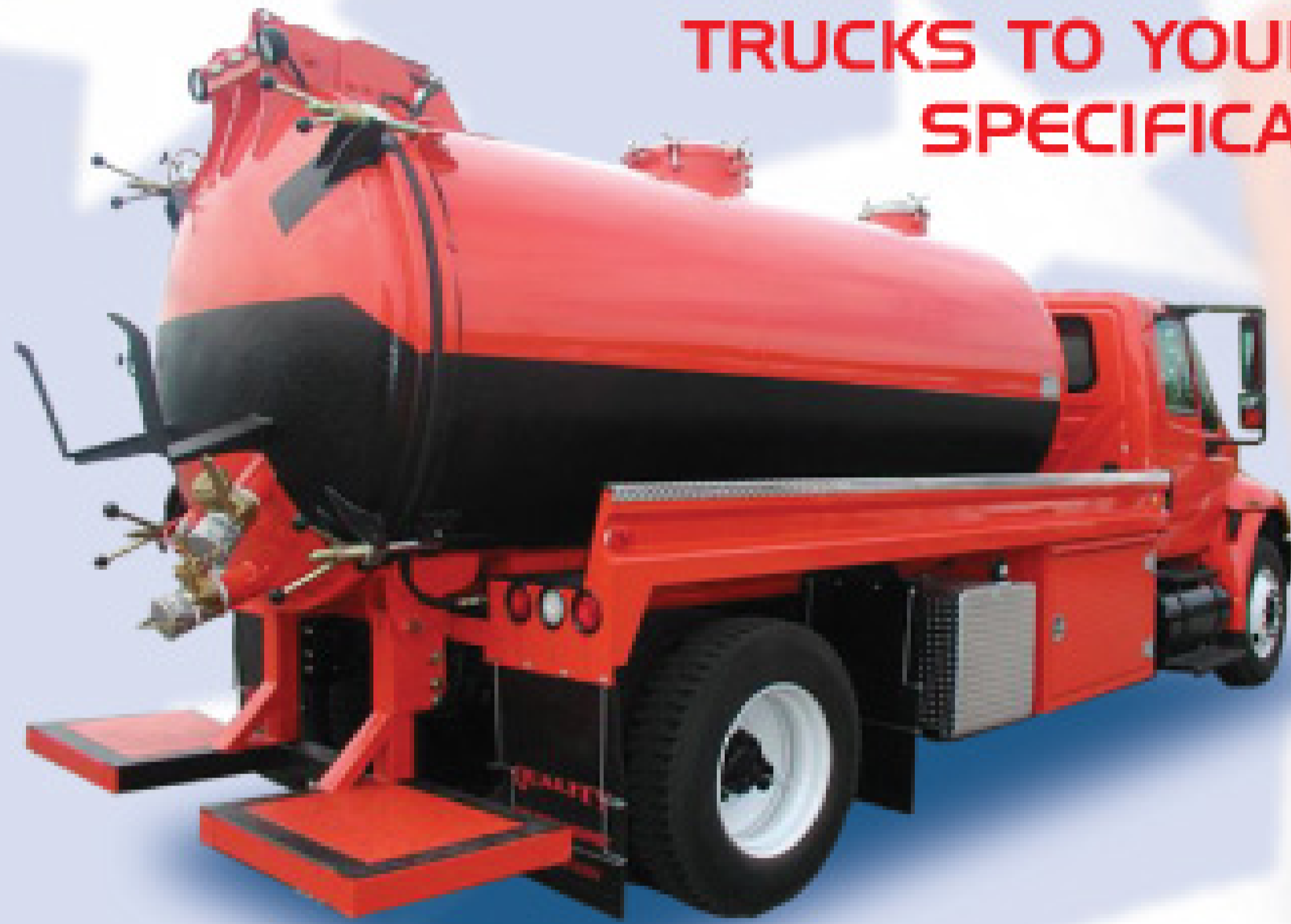
▲ Built for Scott Rowe Septic 2600 gallon full open rear door dump
