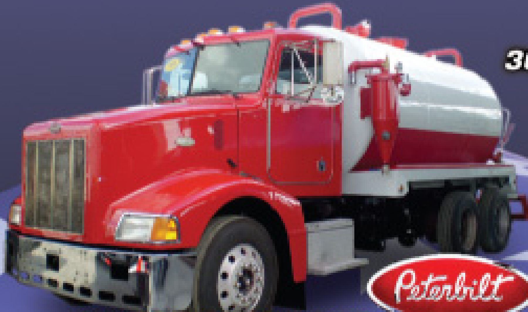
1999 PETERBILT C12 Cat, 10 Spd., 430 HP, 3600 Gallon Carbon Steel Tank, (IN PRODUCTION).
