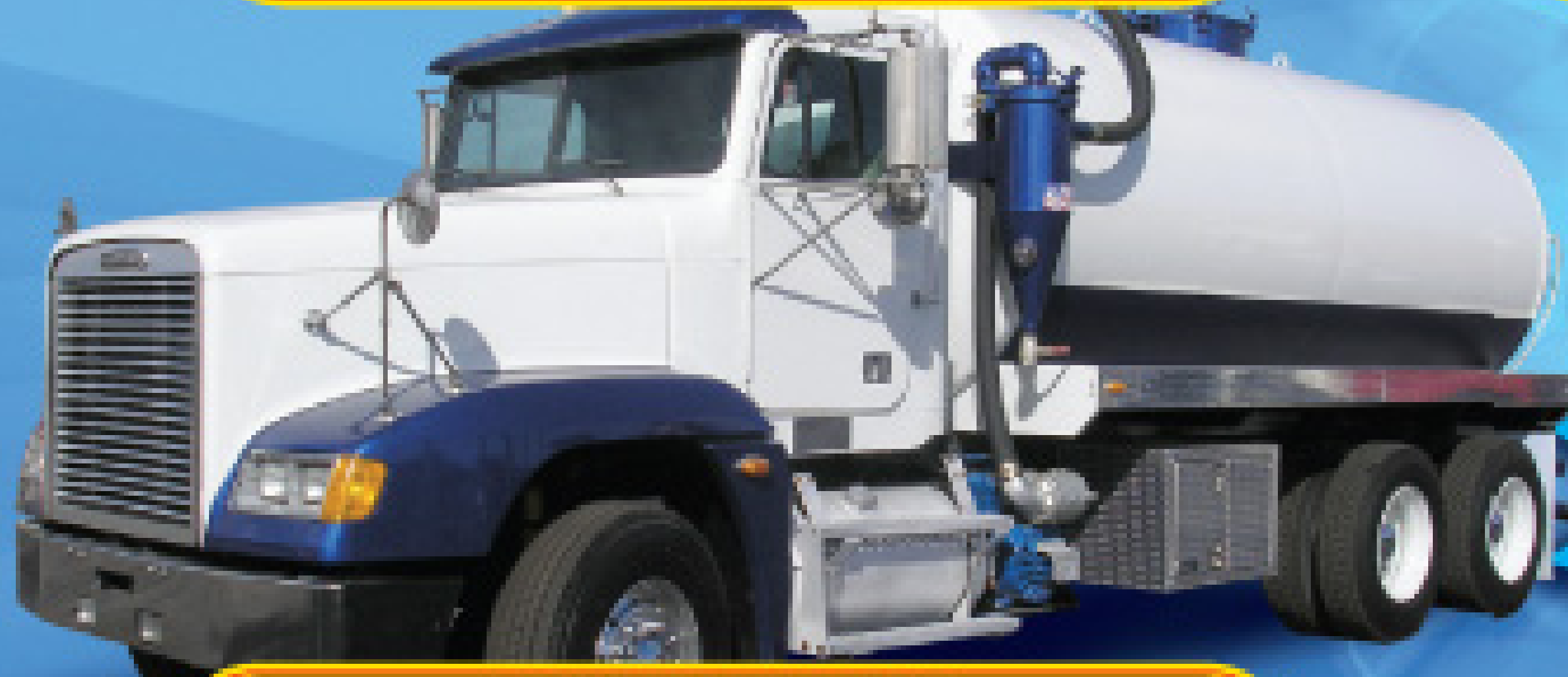
2003 FRTL FLC120 4000 gal US Tanks Double Frame, LC 420 CFM Liquid Cooled
