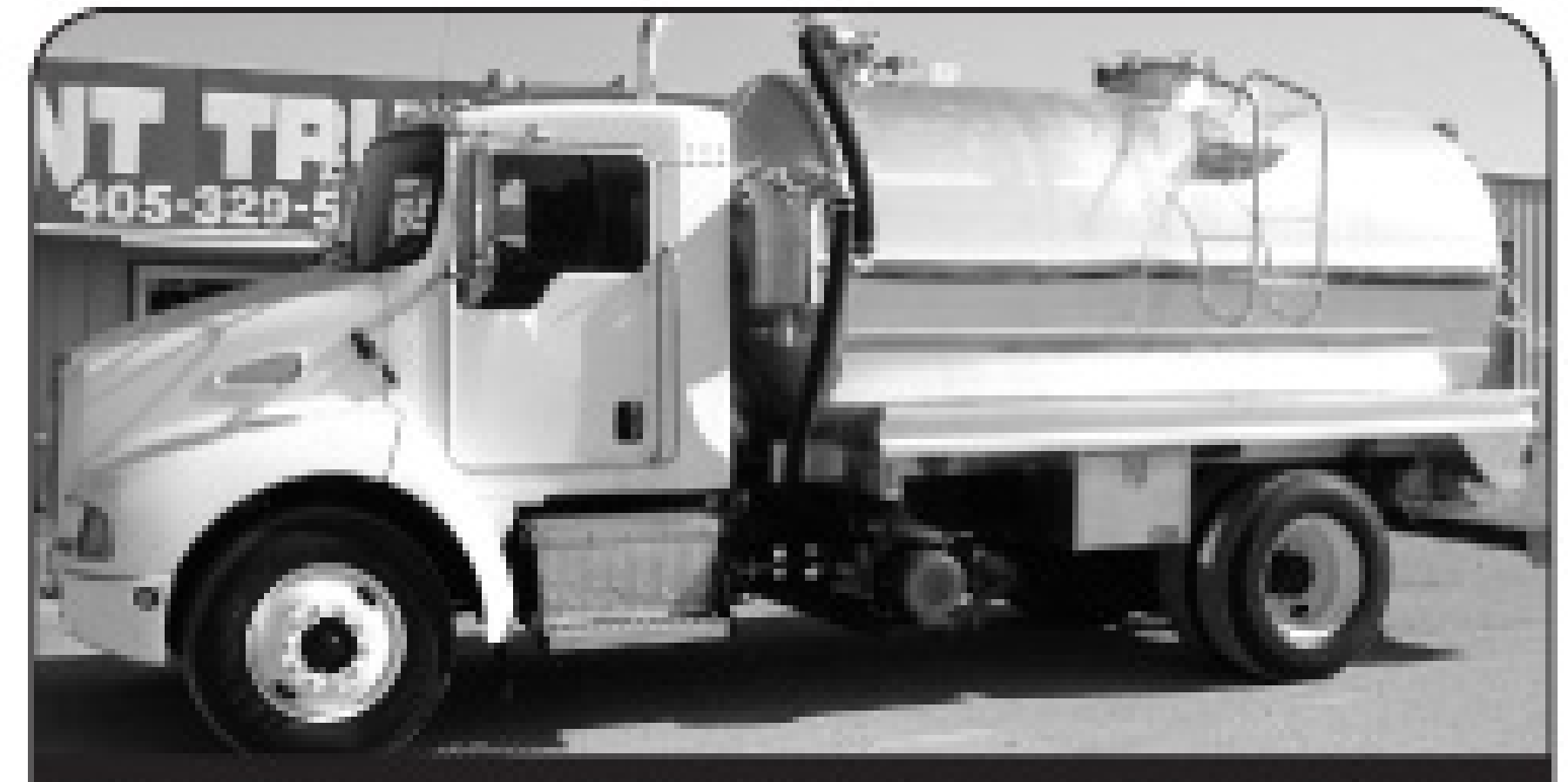
2004 Kenworth T300, Cat C7 (210 hp), 6-spd., 33K GVW, new Wally 753HR (350 cfm), new 2600 gal. aluminum vacuum tank, 2-yr. nationwide drivetrain warranty.
