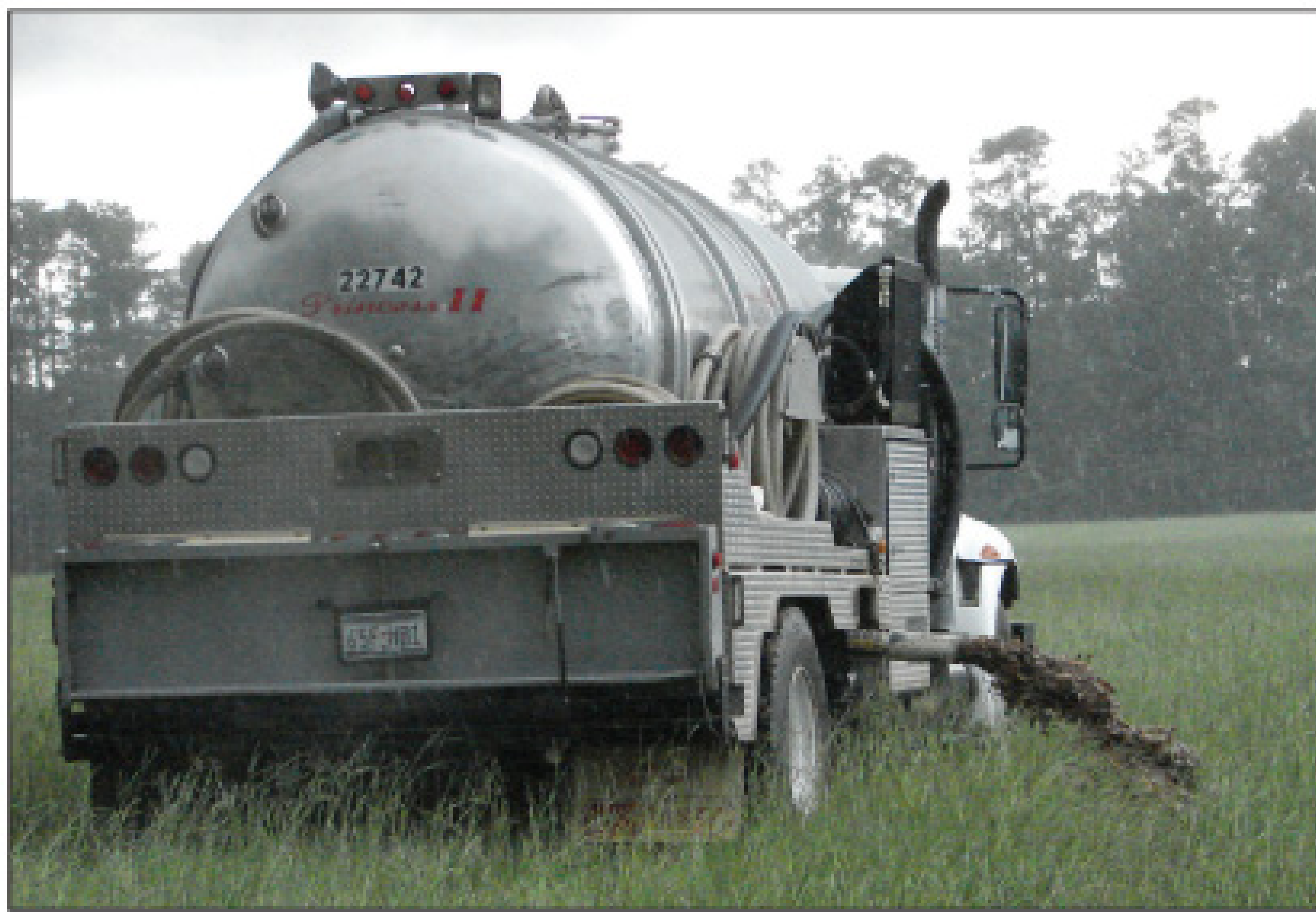
Land application is in progress. In Texas, food crops can't be planted on land where seepage has been spread for 18 months.
