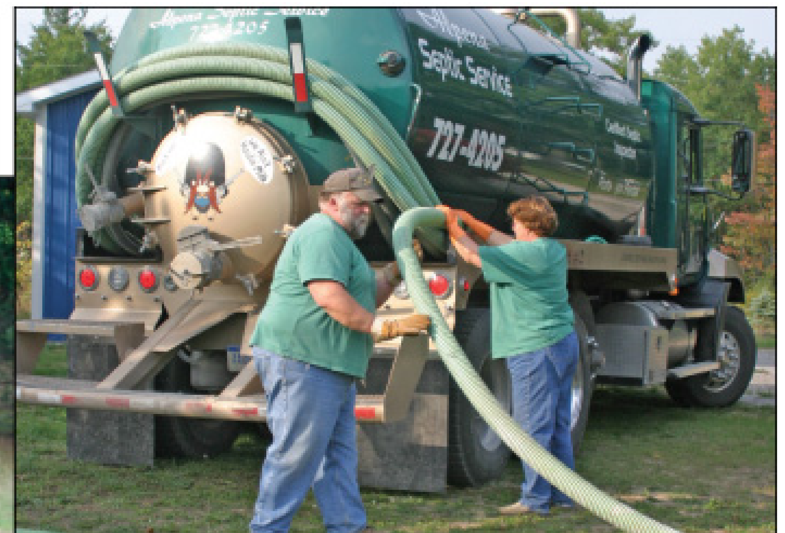
Richard and Lynn Gillespie load vacuum hoses back onto their Mack Vision Series truck after pumping a residential tank in Spruce, Mich.
